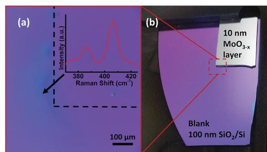
Fig. 5 (a) Contrast-enhanced optical image of the MoS<sub>2</sub> film coated on the SiO<sub>2</sub>/Si substrate, indicating significant contributions from a vapor-phase assisted reaction pathway; arrow indicates the measurement region of the Raman spectrum shown in inset; (b) arrangement of the MoO<sub>3-x</sub>-coated substrate on the blank substrate. The red box represents the region shown in (a).
