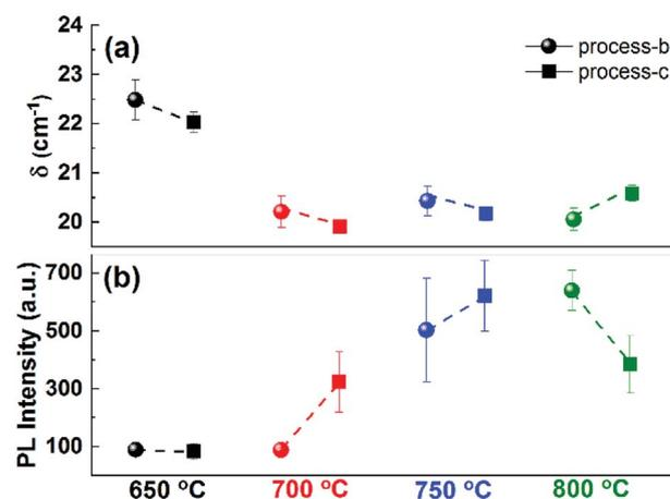
Fig. 2 (a) Raman peak spacing  $\delta$ , and (b) PL intensity for the samples prepared at different processing temperatures, with (process-c), and without (process-b) H<sub>2</sub>S injection delay.
