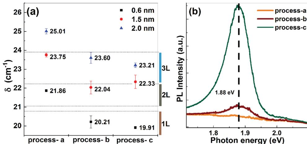
Fig. 1 (a) Peak separation ( $\delta$ ) between Raman modes  $A_{1g}$  and  $E_{2g}^1$  for the samples prepared at 700 °C with different process sequences (process-a/b/c); (b) PL spectra of MoS<sub>2</sub> films produced via different process sequences using 0.6 nm thick MoO<sub>3-x</sub> on Si substrate.
