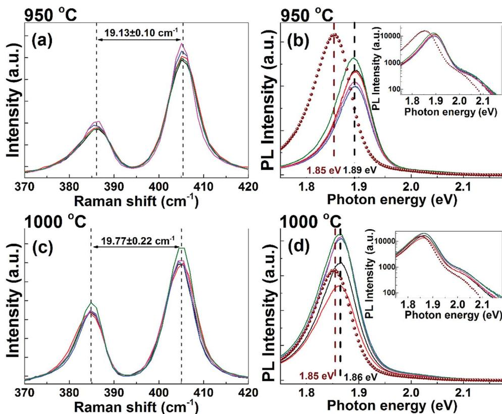
Fig. 3 Raman (a and c) and PL (b and d) spectra of MoS<sub>2</sub> samples prepared at 950 °C (a and b) and 1000 °C (c and d) on SiO<sub>2</sub>/Si. Each graph shows measurements taken at 5 different positions on a 5 mm × 5 mm sample. Results obtained for an exfoliated MoS<sub>2</sub> monolayer flake are shown as dotted lines. Insets in (b and d): PL spectra on a logarithmic scale.
