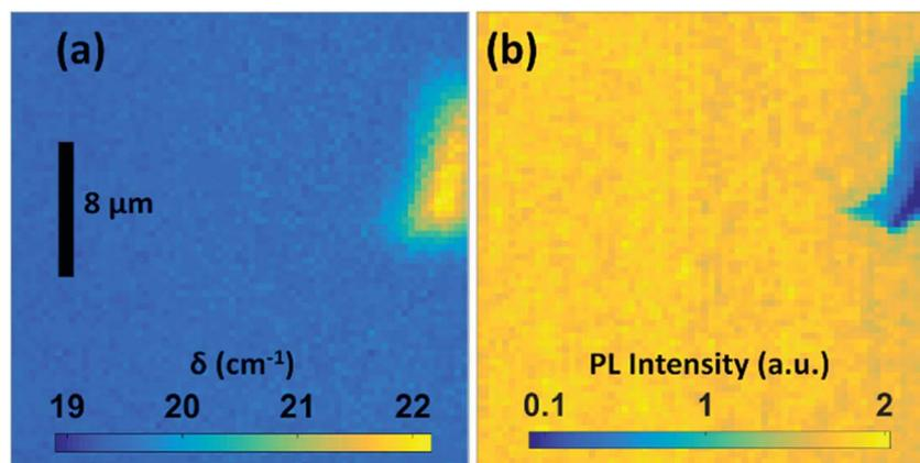
Fig. 4 Spatial map of Raman peak distance (a) and PL (b) recorded on a MoS<sub>2</sub> sample prepared at 950 °C.
