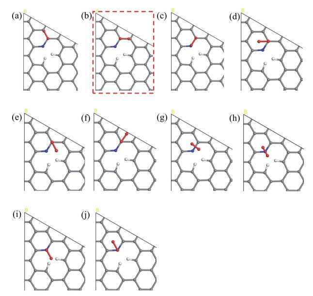
Fig. 2 The potential sites where O<sub>2</sub> can be located on the N6 substrate for the first step of the ORR. N6\_S1\_(a) CBC1 (b) CBC2 (c) CBN (d) CH1 (e) CH2 (f) CH3 (g) HBH (h) HNH (i) NH1 and (j) NH2. The model marked by red dashed line has the lowest energy upon geometry optimization, indicating the most likely adsorption configuration and is used in the free energy diagram.
