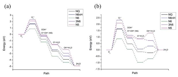
Fig. 4 Free energy diagram at (a)  $U_0 = 0$  V (vs. NHE) and (b) at  $U_{eq} = 1.23$  V (vs. NHE). Reaction pathway is  $O_2$ ,  $O_2^*$ , OOH\*, O\* + H<sub>2</sub>O, OH\* + H<sub>2</sub>O, 2H<sub>2</sub>O.
