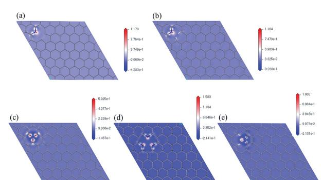
Electron density difference maps with respect to nitrogen atom of (a) N6nH, (b) N6, (c) NQ, (d) 3N6, and (e) N5
