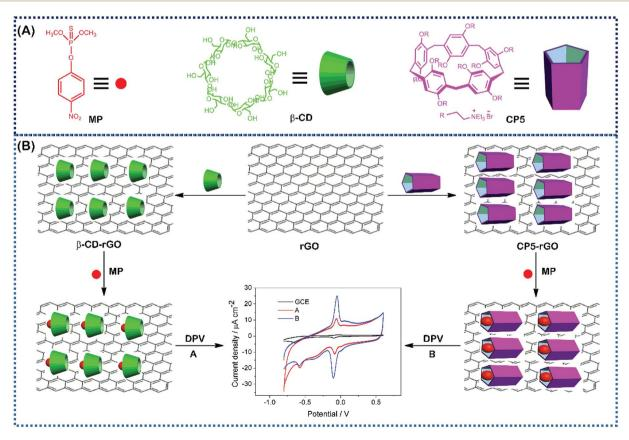
Fig. 1 The corresponding cartoon representations of MP, CP5 and β-CD and the illustration of CP5-rGO (A) and β-CD-rGO (B) nanohybridsbased electrochemical sensing method towards methyl parathion
