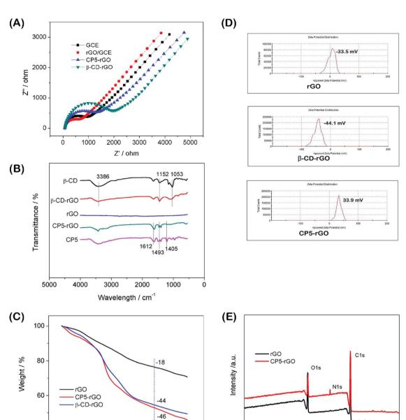
Fig. 3 The EIS characterization of GCE, β-CD-rGO/GCE and CP5-rGO/GCE via [Fe(CN)<sub>6</sub>]<sup>3-/4-</sup> (2.0 mM) redox couple (1:1) with KCl (0.1 M) as supporting electrolyte (A). FTIR spectra of β-CD, β-CD-rGO, rGO, CP5-rGO and CP5 (B). TGA curves of rGO, CP5-rGO and β-CD-rGO (C). Zeta potentials of rGO, β-CD-rGO and CP5-rGO (D). XPS survey spectra of rGO and CP5-rGO (E).
