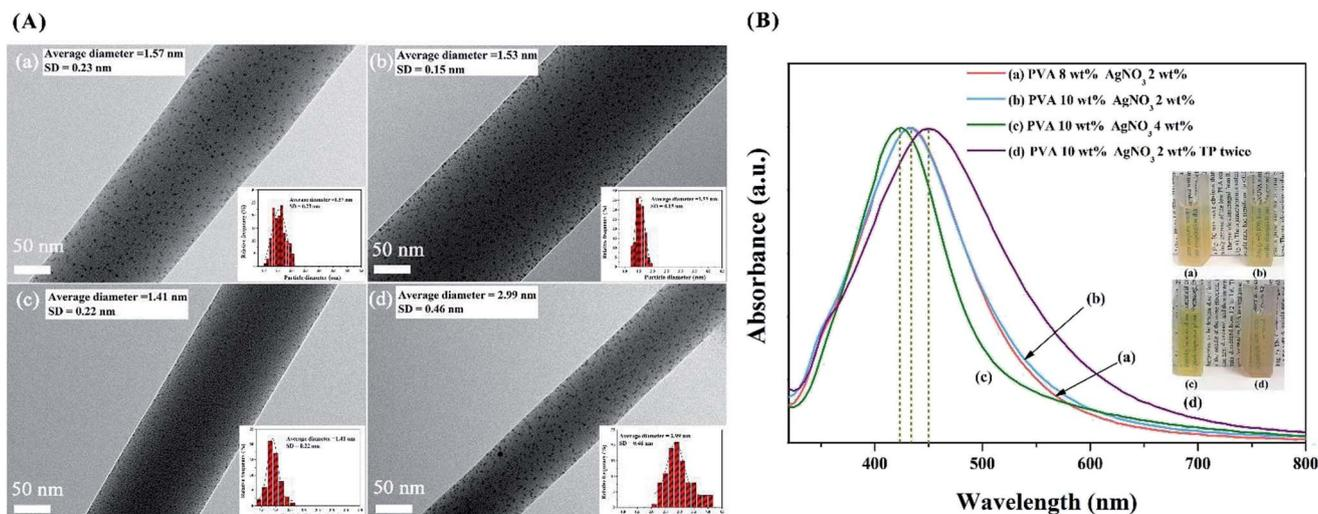
Fig. 10 (A) TEM images of the PVA/Ag NP nanofibres with different average sizes of Ag NPs by changing the solution proportion, (a) PVA 8 wt%, AgNO<sub>3</sub> 2 wt% (relative to the weight of PVA); (b) PVA 10 wt%, AgNO<sub>3</sub> 2 wt%; (c) PVA 10 wt%, AgNO<sub>3</sub> 4 wt%; (d) PVA 10 wt%, AgNO<sub>3</sub> 2 wt%, TP dose twice. (B) UV-vis spectra of Ag NPs in the different reaction systems, and the insets are the photographs of the corresponding Ag NP aqueous solution.<sup>15</sup>
