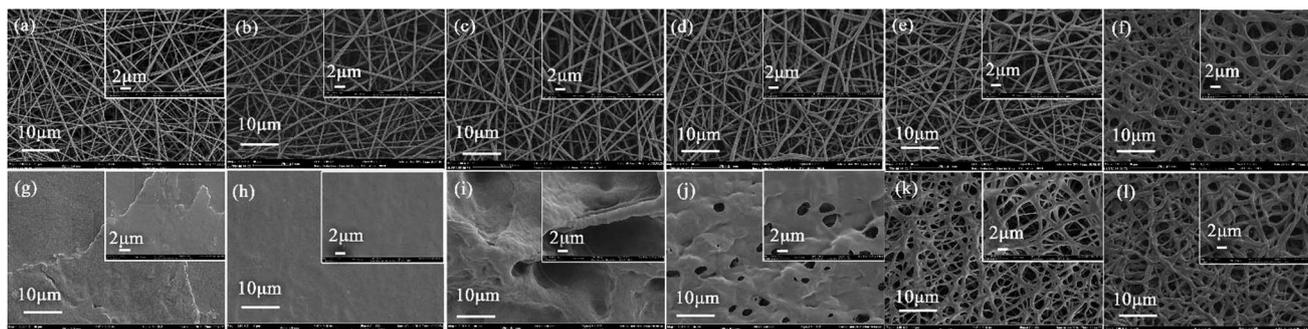
Fig. 12 SEM images of the crosslinked PVA nanofibres at different crosslinking conditions, (a) un-crosslinked; (b) GA 50% (v/v), crosslinked at 30 °C for 24 h; (c) GA 25% (v/v), crosslinked at 60 °C for 24 h; (d) GA 25% (v/v), crosslinked at 30 °C for 24 h; (e) GA 25% (v/v), crosslinked at 30 °C for 48 h; (f) GA 25% (v/v), crosslinked at 30 °C for 72 h. (g)–(l) The corresponding samples immersed in water for 48 h.
