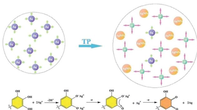
Fig. 3 Schematic illustration of the mechanism for the change of the Ag NP aqueous solution conductivity.
