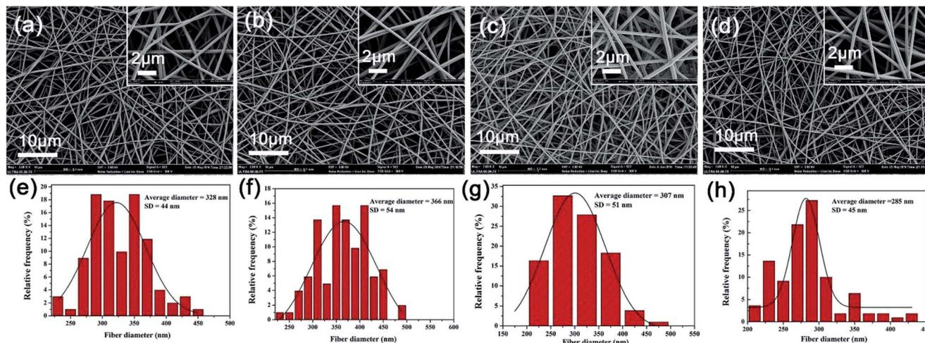
Fig. 7 SEM images of the (a) neat PVA; (b) PVA/TP; (c) PVA/AgNO<sub>3</sub>; and (d) PVA/Ag NP nanofibers. The corresponding diameter distributions of (e) neat PVA; (f) PVA/TP; (g) PVA/AgNO<sub>3</sub>; and (h) PVA/Ag NP nanofibers.
