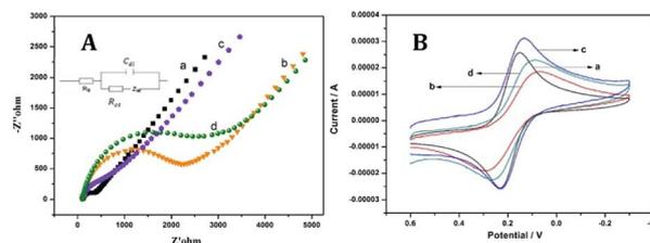
Fig. 2 (A) EIS and (B) CV curves of (a) bare GCE, (b) FDU-15/GCE, (c) AuNPs/FDU-15/GCE and (d) PPO/AuNPs/FDU-15/GCE in PBS buffer solution containing 1.0 mM  $[\text{Fe}(\text{CN})_6]^{4-/3-}$  and 0.1 M of KCl.
