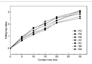
Fig. 2 Effect of contact time on antibiotic-resistant bacteria disinfection by  ${\rm ClO}_2$ .
