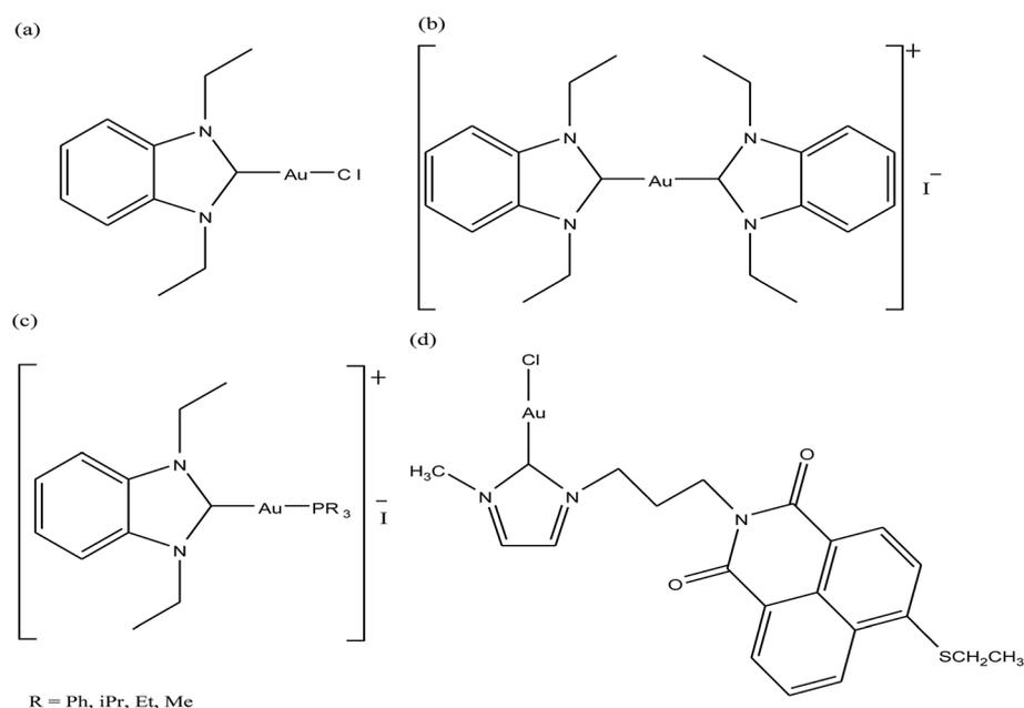
Fig. 31 Chemical structures of (a)  $[\text{Au}(\text{NHC})\text{Cl}]$ , (b)  $[\text{Au}(\text{NHC})_2]\text{I}$  (c)  $[\text{Au}(\text{NHC})\text{PR}_3]\text{I}$  and (d)  $[\text{Au}(\text{NHC})(\text{NAP})\text{Cl}]$  complexes.
