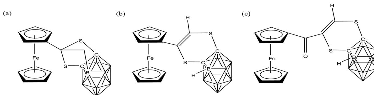
Fig. 52 Chemical structures of the ferrocene-carborane conjugates (a)  $[\text{Fe}(\eta^5\text{-cp})_2(\text{SB1})]$ , (b)  $[\text{Fe}(\eta^5\text{-cp})_2(\text{SB2})]$  and (c)  $[\text{Fe}(\eta^5\text{-cp})_2(\text{SBCO})]$ .
