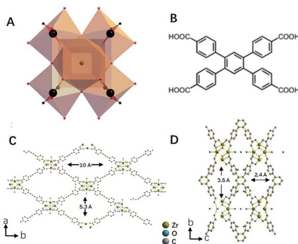
Fig. 1 Crystal structure of Zr-CAU-24 that is constructed from the  $[\text{Zr}_6(\mu_3\text{-O})_4(\mu_3\text{-OH})_4]^{12+}$  clusters (A) and  $\text{TCPB}^{4-}$  molecules (B). Ball-stick models of Zr-CAU-24 crystals (C) and (D).
