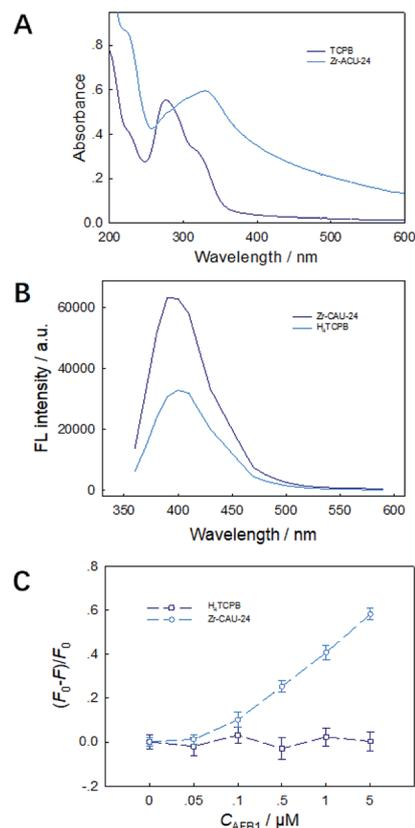
**Fig. 4** UV-visible spectrum (A) and emission spectra ( $\lambda_{\text{em}} = 410$  nm) (B) of TCPB<sup>4+</sup> molecules and Zr-CAU-24 crystals. FL intensity fading of Zr-CAU-24 crystals and TCPB<sup>4+</sup> molecules with the existence of AFB1 (C).
