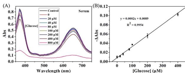
Fig. 5 The absorption spectra of the  $\text{KMnO}_4$ -TMB system for analyzing diluted serum with addition of different concentrations of glucose (0, 20, 40, 80, 100, 200, 400 and 800  $\mu\text{M}$ , respectively). (B) Calibration curve of glucose sensing in diluted serum using the reduced absorbance intensity ( $-\Delta\text{Abs}$ ) as the ordinate and the concentrations of added glucose as the abscissa. The data shown here represent the average of three independent experiments.
