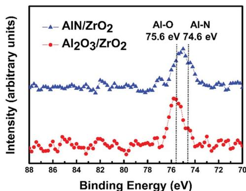
Fig. 3 Al 2p XPS spectra of the  $\text{Al}_2\text{O}_3/\text{ZrO}_2$  and  $\text{AlN}/\text{ZrO}_2$  gate stacks. The Al–O (75.6 eV) and Al–N (74.6 eV) bonds were present in the  $\text{Al}_2\text{O}_3/\text{ZrO}_2$  and  $\text{AlN}/\text{ZrO}_2$  samples.
