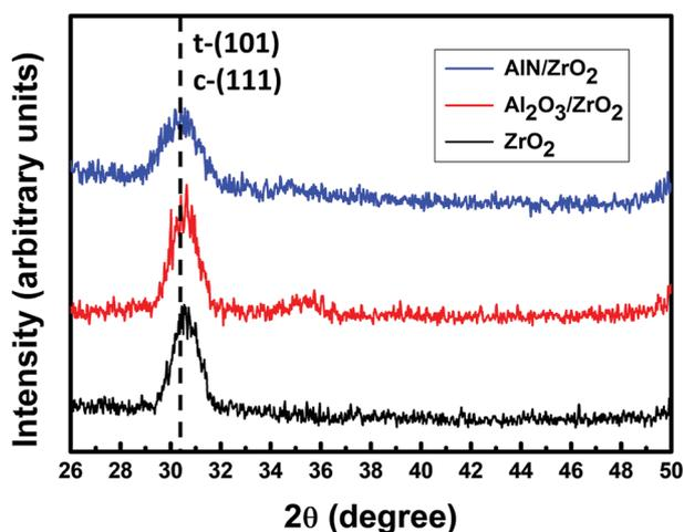
Fig. 5 GIXRD patterns of  $\text{ZrO}_2$ ,  $\text{Al}_2\text{O}_3/\text{ZrO}_2$ , and  $\text{AlN}/\text{ZrO}_2$  gate stacks. The obvious diffraction peak at  $2\theta = 30.4^\circ$  is associated with tetragonal/cubic  $\text{ZrO}_2$ .
