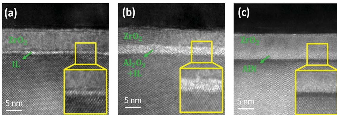
Fig. 4 Cross-sectional HRTEM images of the (a)  $\text{ZrO}_2$ , (b)  $\text{Al}_2\text{O}_3/\text{ZrO}_2$ , and (c)  $\text{AlN}/\text{ZrO}_2$  gate stacks. There is a sharp interface between  $\text{AlN}$  and  $\text{Ge}$  in the  $\text{AlN}/\text{ZrO}_2$  sample.
