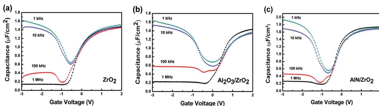
**Fig. 8** The frequency dependence of the  $C$ - $V$  curves of the (a)  $\text{ZrO}_2$ , (b)  $\text{Al}_2\text{O}_3/\text{ZrO}_2$ , and (c)  $\text{AlN}/\text{ZrO}_2$  gate stacks. Low-frequency dispersion was observed in the  $\text{AlN}/\text{ZrO}_2$  sample.
