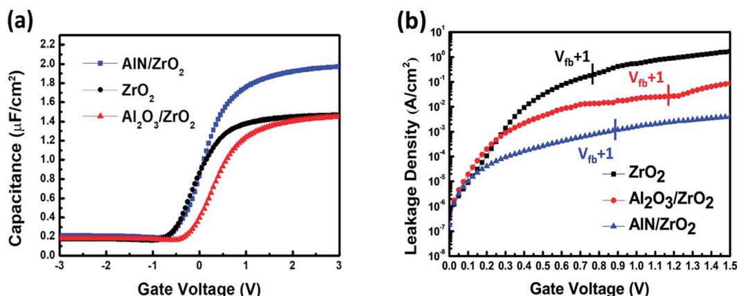
Fig. 6 (a)  $C$ - $V$  and (b)  $I$ - $V$  characteristics of the  $\text{ZrO}_2$ ,  $\text{Al}_2\text{O}_3/\text{ZrO}_2$ , and  $\text{AlN}/\text{ZrO}_2$  gate stacks. The  $\text{AlN}/\text{ZrO}_2$  gate stack had a higher capacitance and a lower  $J_g$  than the  $\text{ZrO}_2$  or  $\text{Al}_2\text{O}_3/\text{ZrO}_2$  samples.
