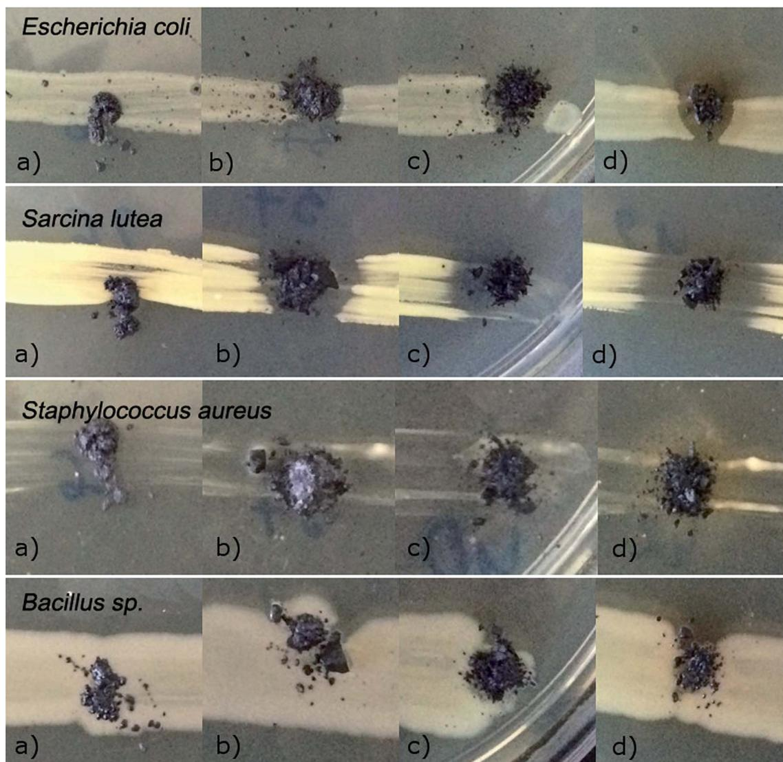
Fig. 5 Growth of *Escherichia coli*, *Sarcina lutea*, *Staphylococcus aureus*, and *Bacillus sp.* bacteria strains in the presence of  $\text{Ti}_3\text{C}_2$  MXene (a),  $\text{Ti}_3\text{C}_2/\text{Al}_2\text{O}_3/\text{Ag}$  (b),  $\text{Ti}_3\text{C}_2/\text{SiO}_2/\text{Ag}$  (c), and  $\text{Ti}_3\text{C}_2/\text{SiO}_2/\text{Pd}$  (d) nanocomposite structures.
