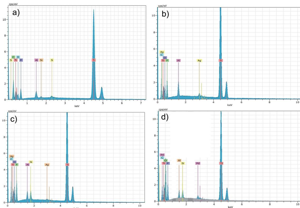
Fig. 2 Results of EDS analysis obtained for the  $\text{Ti}_3\text{C}_2$  MXene (a) as well as:  $\text{Ti}_3\text{C}_2/\text{Al}_2\text{O}_3/\text{Ag}$  (b),  $\text{Ti}_3\text{C}_2/\text{SiO}_2/\text{Ag}$  (c),  $\text{Ti}_3\text{C}_2/\text{SiO}_2/\text{Pd}$  (d) nanocomposites.
