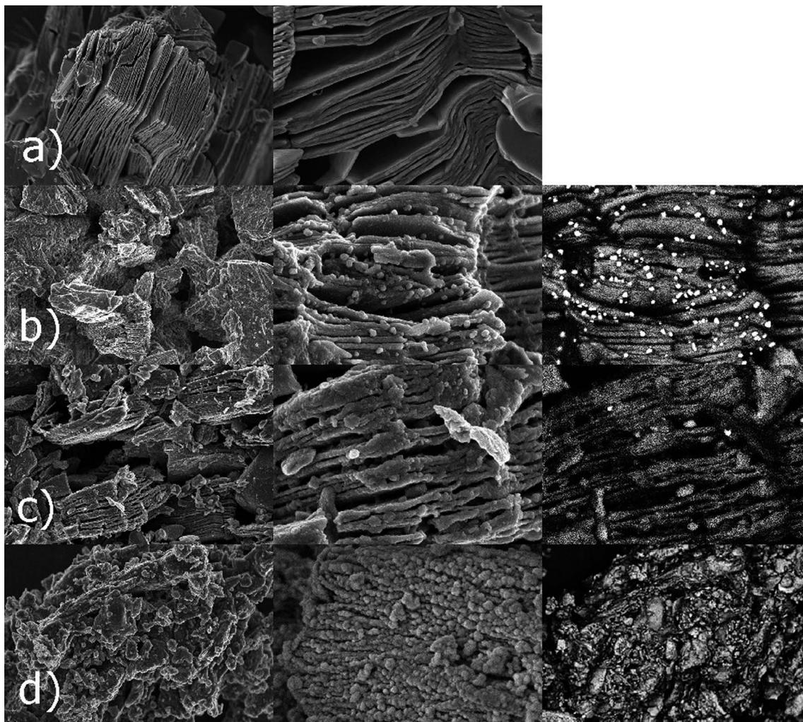
Fig. 1 SEM images obtained for the  $\text{Ti}_3\text{C}_2$  MXene (a),  $\text{Ti}_3\text{C}_2/\text{Al}_2\text{O}_3/\text{Ag}$  (b),  $\text{Ti}_3\text{C}_2/\text{SiO}_2/\text{Ag}$  (c), and  $\text{Ti}_3\text{C}_2/\text{SiO}_2/\text{Pd}$  (d) nanocomposites.
