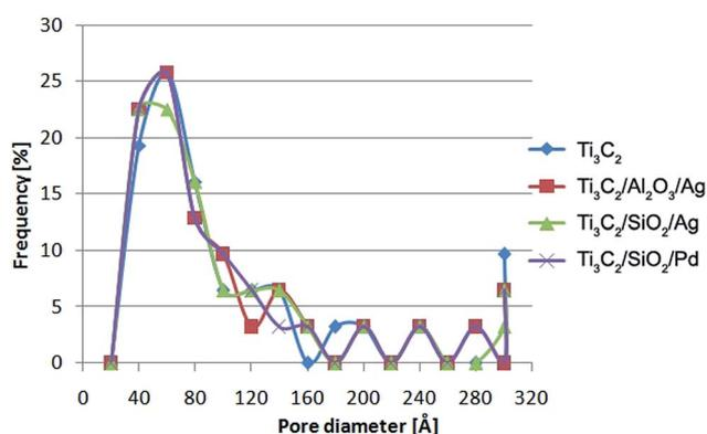
**Fig. 4** The distributions of pore diameter obtained using BJH method for the  $\text{Ti}_3\text{C}_2$  MXene,  $\text{Ti}_3\text{C}_2/\text{Al}_2\text{O}_3/\text{Ag}$ ,  $\text{Ti}_3\text{C}_2/\text{SiO}_2/\text{Ag}$ , and  $\text{Ti}_3\text{C}_2/\text{SiO}_2/\text{Pd}$  nanocomposites.
