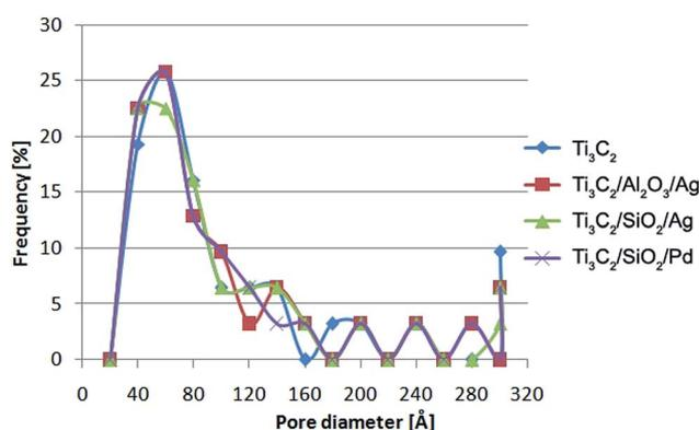
**Fig. 4** The distributions of pore diameter obtained using BJH method for the  $\text{Ti}_3\text{C}_2$  MXene,  $\text{Ti}_3\text{C}_2/\text{Al}_2\text{O}_3/\text{Ag}$ ,  $\text{Ti}_3\text{C}_2/\text{SiO}_2/\text{Ag}$ , and  $\text{Ti}_3\text{C}_2/\text{SiO}_2/\text{Pd}$  nanocomposites.
