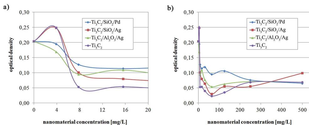
Fig. 6 Antibacterial impact of  $\text{Ti}_3\text{C}_2$  MXene,  $\text{Ti}_3\text{C}_2/\text{Al}_2\text{O}_3/\text{Ag}$ ,  $\text{Ti}_3\text{C}_2/\text{SiO}_2/\text{Ag}$ , and  $\text{Ti}_3\text{C}_2/\text{SiO}_2/\text{Pd}$  nanocomposite against *Staphylococcus aureus* bacteria. The results are presented in the range of  $0\text{--}20\text{ mg l}^{-1}$  (a), and  $0\text{--}500\text{ mg l}^{-1}$  (b) of nanomaterial concentration.
