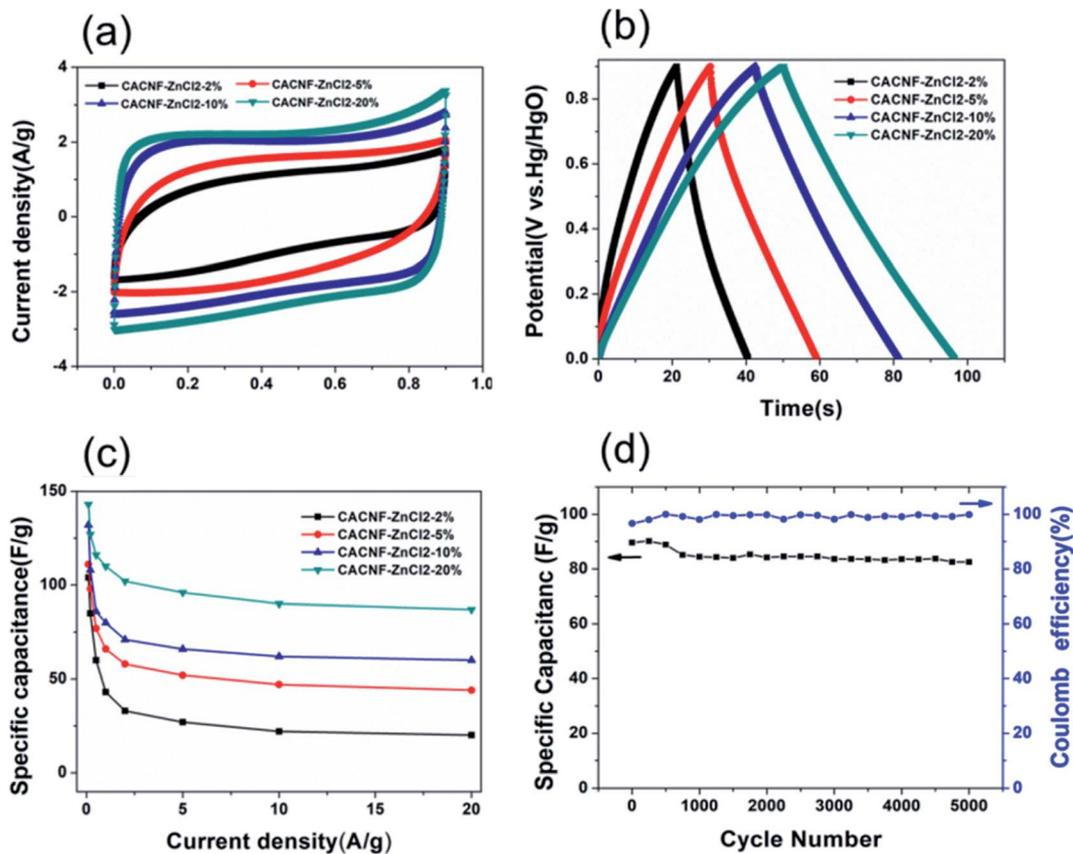
Fig. 7 Electrochemical performance from two-electrode test in 6 M KOH. (a) CV curves at  $5 \text{ mV s}^{-1}$ ; (b) galvanostatic charge/discharge curves at  $1 \text{ A g}^{-1}$ ; (c) specific capacitance at different current densities; (d) cycling stability of CACNF-ZnCl<sub>2</sub>-20% at  $5 \text{ A g}^{-1}$ .
