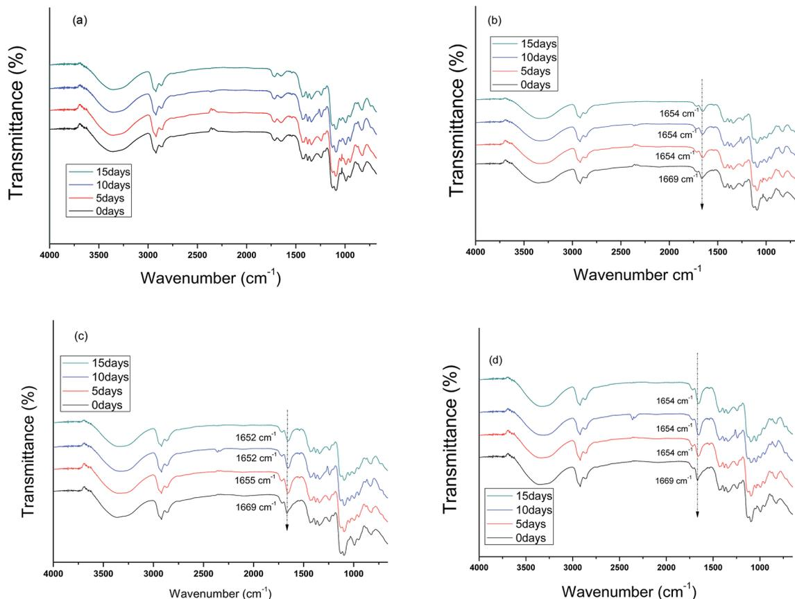
Fig. 2 The FTIR spectra on different days after immersion of (a) PVAm0, (b) PVAm0.5, (c) PVAm1.0 and (d) PVAm1.5 membranes in the 50 : 30 : 20 ECH/IPA/water (w/w) feed mixture solution at 60 °C.
