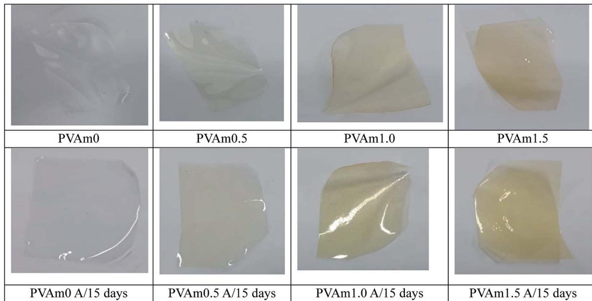
Fig. 6 Physical status of the membranes after 15 days of immersion in the ECH/IPA/water (50 : 30 : 20, w/w) feed mixture solution at 60 °C.
