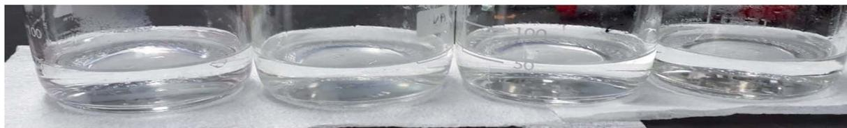
Fig. 5 Clarity of the 50 : 30 : 20 ECH/IPA/water (w/w) feed mixture solution after 15 days of immersion.
