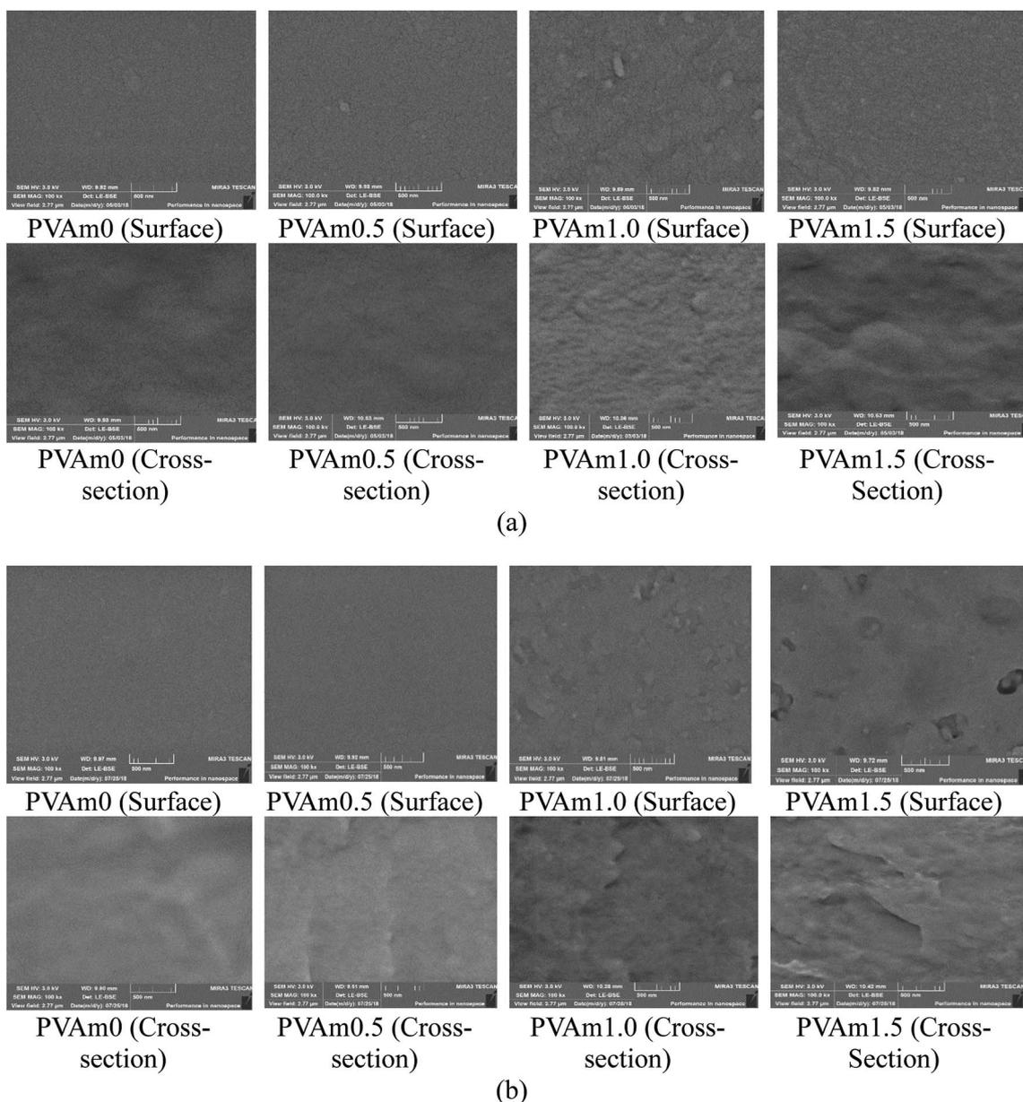
Fig. 3 SEM micrographs of the PVAm0, PVAm0.5, PVAm1.0, and PVAm1.5 membranes (a) before and (b) after immersion in the 50 : 30 : 20 ECH/IPA/water (w/w) feed mixture solution at 60 °C.
