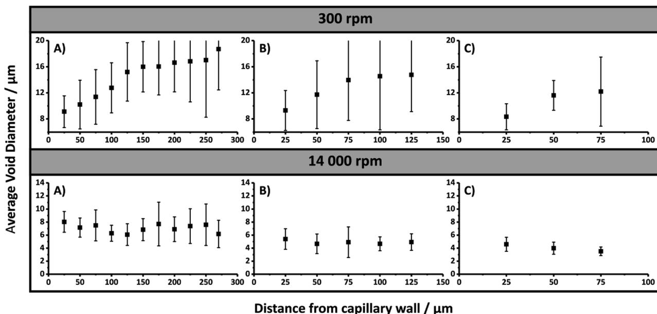
Fig. 3 Plot of average void diameter with increased distance from capillary wall for poly(HIPE)s prepared with emulsification at 300 or 14 000 rpm within different capillary i.d.s: (A) 540  $\mu\text{m}$ ; (B) 250  $\mu\text{m}$ ; (C) 150  $\mu\text{m}$ .
