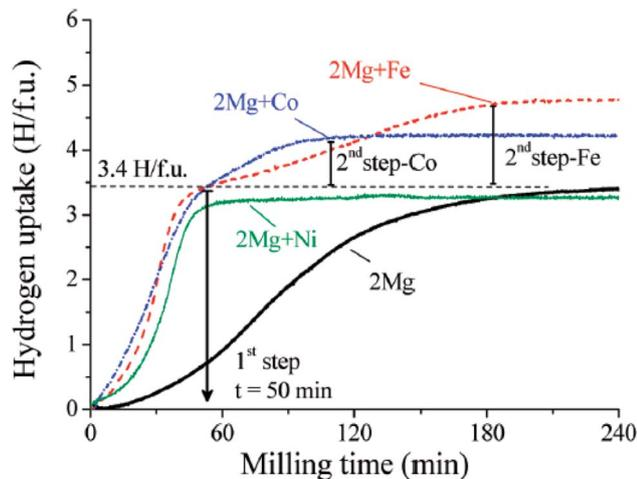
Fig. 6 Absorbed hydrogen atoms by formula unit of the formed hydride during RBM of Mg and  $Mg^{+2}TM$  mixtures (TM = Ni, Fe, and Co) (The number of absorbed H atoms per unit metal or alloy formula (H/f.u.)).<sup>38</sup>
