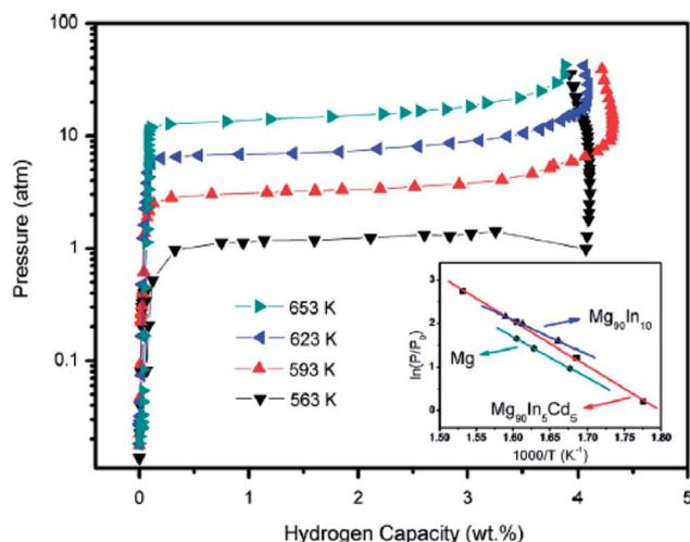
Fig. 8 PCT and van't Hoff plot (the inset) for the hydrogen desorption of the Mg<sub>90</sub>In<sub>5</sub>Cd<sub>5</sub> alloy.<sup>47</sup>
