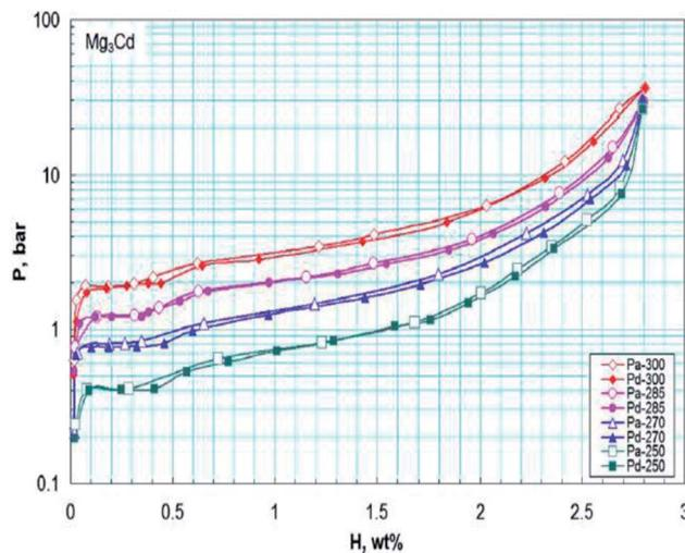
Fig. 7 PCT diagrams of the studied  $Mg_3Cd$  alloy in the temperature range of 250–300 °C. The open and filled symbols correspond to the absorption and desorption branches of the curves, respectively.<sup>42</sup>
