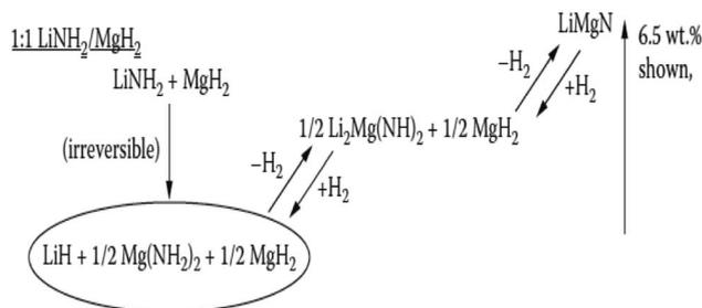
Fig. 24 Mechanism for hydrogen absorption/desorption of 1 : 1 LiNH<sub>2</sub>/MgH<sub>2</sub>.<sup>102</sup>
