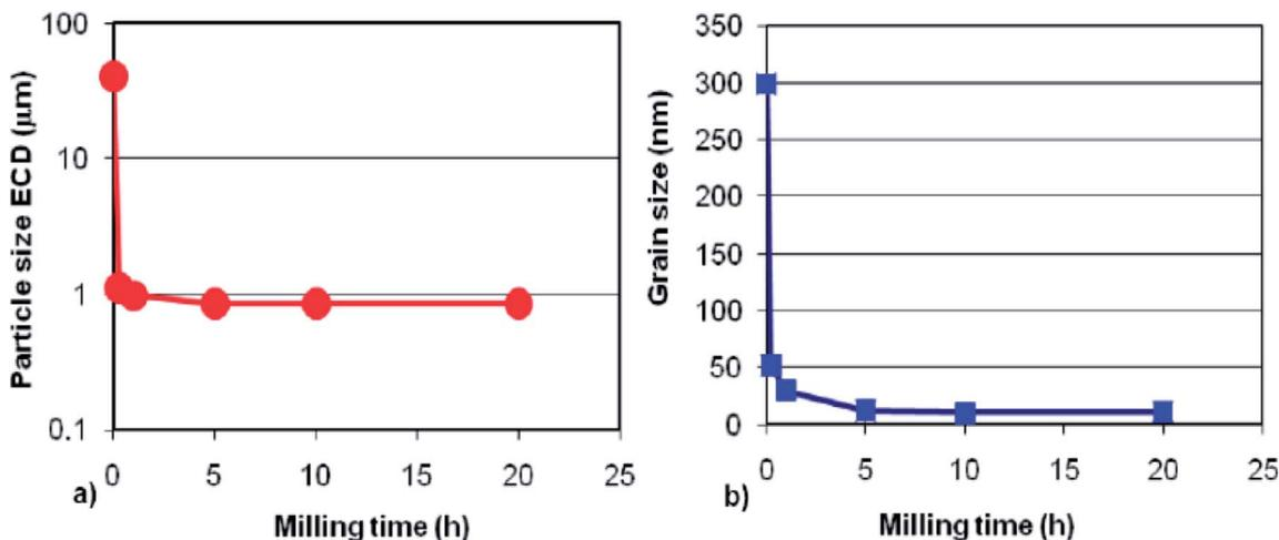
Fig. 4 Simultaneous reduction in the (a) particle size and (b) grain size as a function of ball milling time of  $\text{MgH}_2$ .<sup>26</sup>
