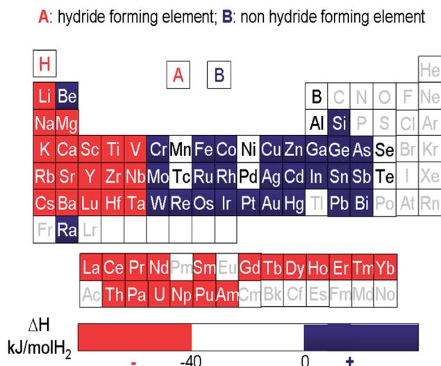
Fig. 5 Hydride and non-hydride forming elements in the periodic table of elements.<sup>28</sup>
