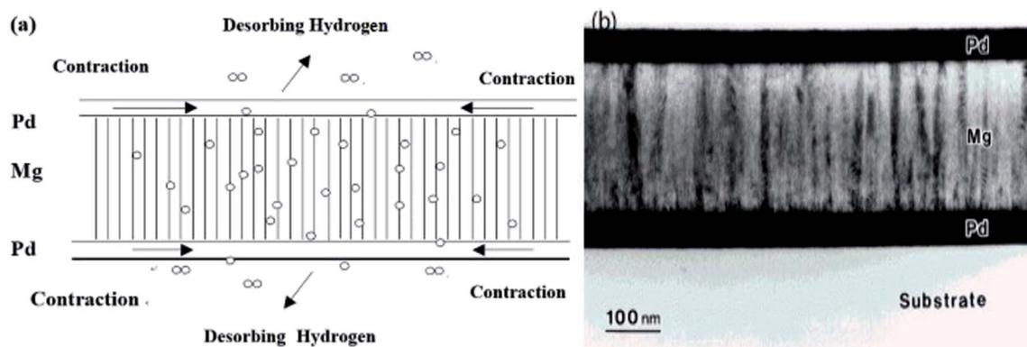
Fig. 16 Schematic representation of the co-operative phenomenon (a) and TEM micrographs of the cross-section of Pd (50 nm)/Mg (200 nm)/Pd (50 nm) films before hydrogenation (b).<sup>61,62</sup>
