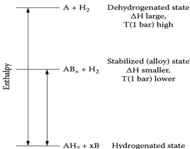
Fig. 22 Generalized enthalpy diagram illustrating destabilization through alloy formation upon dehydrogenation.<sup>89</sup>
