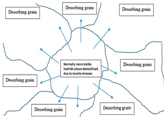
Fig. 25 Schematic representation of the potential synergistic effects observed in multiphase powders.<sup>70</sup>
