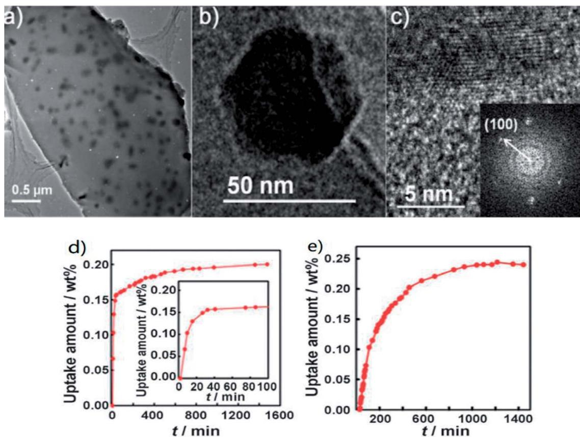
Fig. 26 High-resolution transmission electron microscopy (HRTEM) images of (a) Mg@SNU-9'b, (b) hexagonal-shaped Mg nanocrystal and (c) its edge image showing the lattice fringe (100) *d*-spacing of Mg<sup>0</sup> (2.7782 Å, JCPDS 04-0770). Inset: selected-area electron diffraction (SAED) pattern. H<sub>2</sub> absorption kinetics of Mg@SNU-9'b at (d) 325 K and 80 bar and (e) 415 K and 40 bar.<sup>124</sup>
