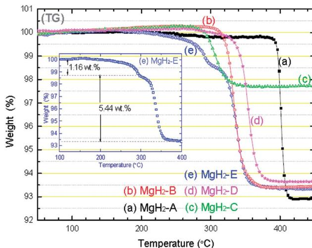
Fig. 20 TG-DTA curves of (a)  $\text{MgH}_2\text{-A}$ , (b)  $\text{MgH}_2\text{-B}$ , (c)  $\text{MgH}_2\text{-C}$ , (d)  $\text{MgH}_2\text{-D}$ , and (e)  $\text{MgH}_2\text{-E}$  samples. The heating rate was  $2 \text{ }^\circ\text{C min}^{-1}$  from room temperature to  $450 \text{ }^\circ\text{C}$  in each case. The inset shows the detail of the mass loss profile for  $\text{MgH}_2\text{-E}$ .<sup>83</sup>
