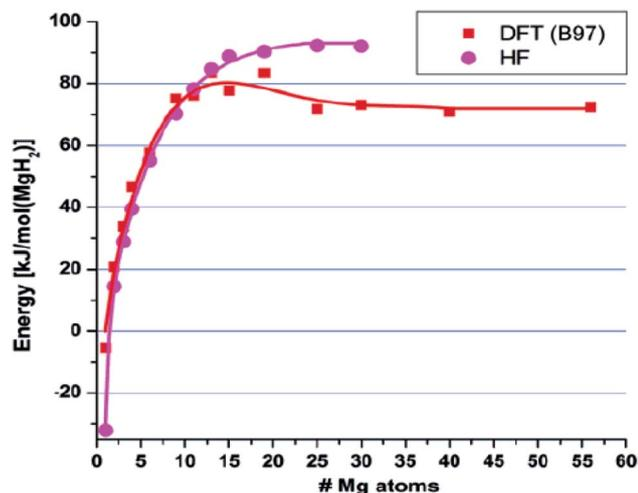
Fig. 10 Calculated desorption energies for  $\text{MgH}_2$  clusters using both the HF method and DFT method (B97 functional). The energies were normalized per mole of  $\text{H}_2$  released.<sup>50</sup>
