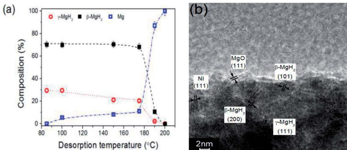
Fig. 21 Thermal stability of  $\gamma$ -MgH<sub>2</sub> during hydrogen desorption as function of desorption temperature (a) and HRTEM images of electro-synthesized Mg after hydrogen absorption at 100 °C (b).<sup>85</sup>
