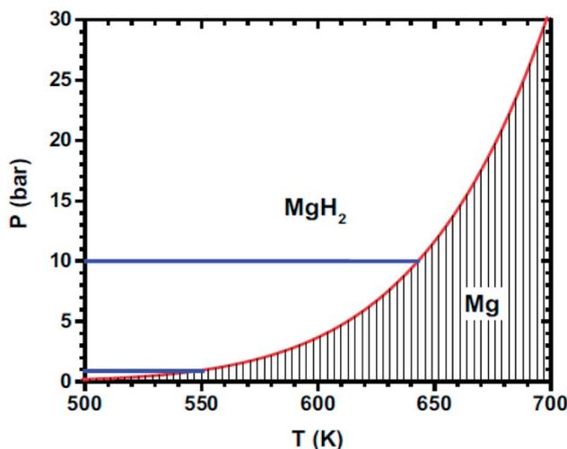
Fig. 2 Temperature dependence of the dissociation pressure of MgH<sub>2</sub>.<sup>14</sup>
