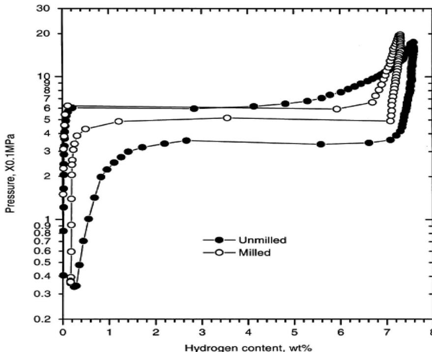
Fig. 3 Pressure-composition-temperature (PCT) curves of the unmillied and ball-milled  $\text{MgH}_2$  at 623 K.<sup>25</sup>
