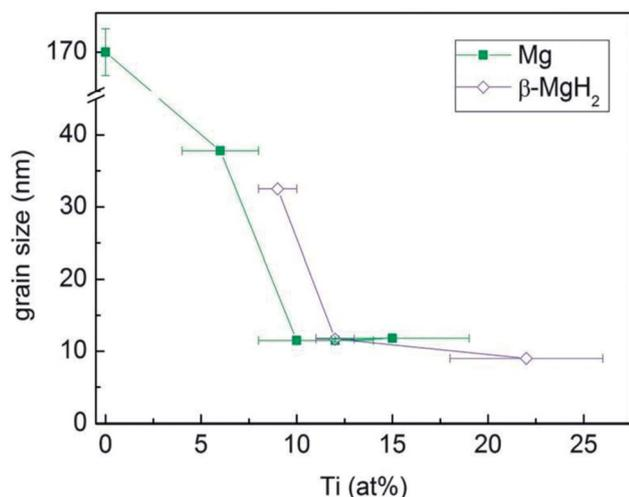
Fig. 13 Mean crystallite size of the Mg and  $\beta$ -MgH<sub>2</sub> phases in the Mg–Ti and Mg–Ti–H samples as a function of Ti content.<sup>56</sup>
