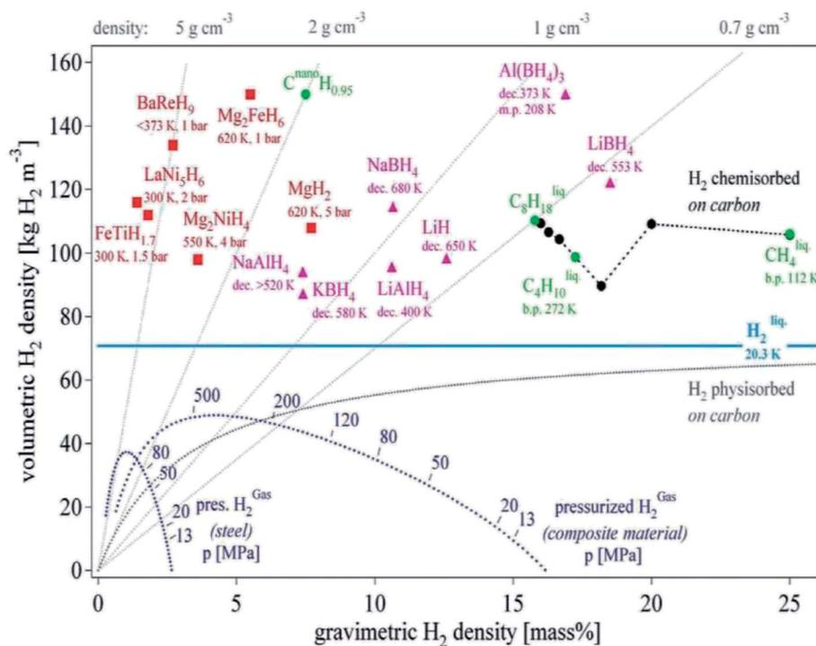
Fig. 1 Gravimetric and volumetric hydrogen density of various hydrogen storage materials.<sup>5</sup>
