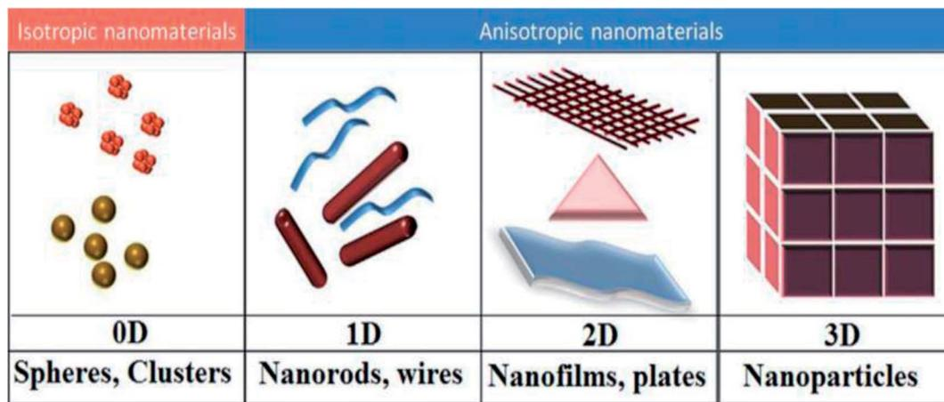
Fig. 9 Schematic representation of the various dimensions (0D, 1D, 2D, and 3D) of nanomaterials.<sup>48</sup>
