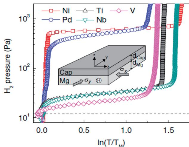
Fig. 17 Effect of cap layer: PTI measured at 333 K for Ti(10 nm)/Mg(20 nm)/X(10 nm)/Pd(10 nm) samples deposited on glass with X = Ni, Pd, Ti, Nb, and V.<sup>67</sup>
