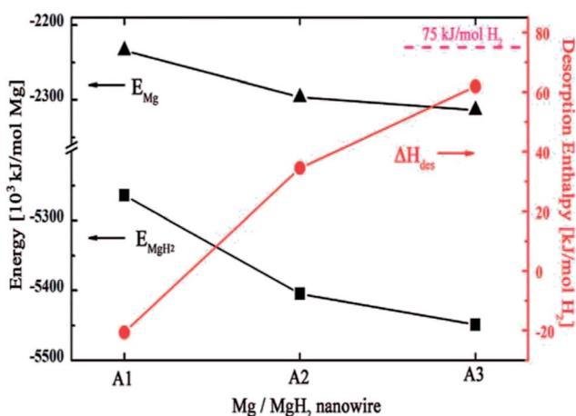
Fig. 15 Desorption enthalpy for MgH<sub>2</sub> nanowires (red line) and the size effect of the calculated energies for magnesium (triangle) and MgH<sub>2</sub> (tetragon) nanowires.<sup>60</sup>
