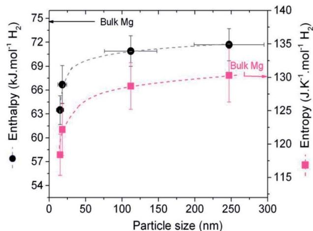
Fig. 11 Evolution of  $\Delta H$  and  $\Delta S$  versus size of the magnesium nanoparticles. The dotted line is a guide to the eyes.<sup>51</sup>
