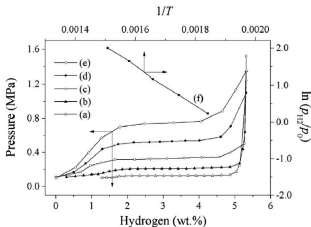
Fig. 12 Dehydrogenation isotherms of the material from Mg and C in a ratio of 70 : 30, milled for 3 h under 1 MPa H<sub>2</sub> at 543 K (a), 573 K (b), 603 K (c), 633 K (d), and 663 K (e), and plot of  $\ln(P_{\text{H}_2}/P_0)$  versus  $1/T$  (f).<sup>55</sup>
