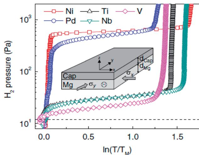
Fig. 17 Effect of cap layer: PTI measured at 333 K for Ti(10 nm)/Mg(20 nm)/Pd(10 nm) samples deposited on glass with X = Ni, Pd, Ti, Nb, and V.<sup>67</sup>
