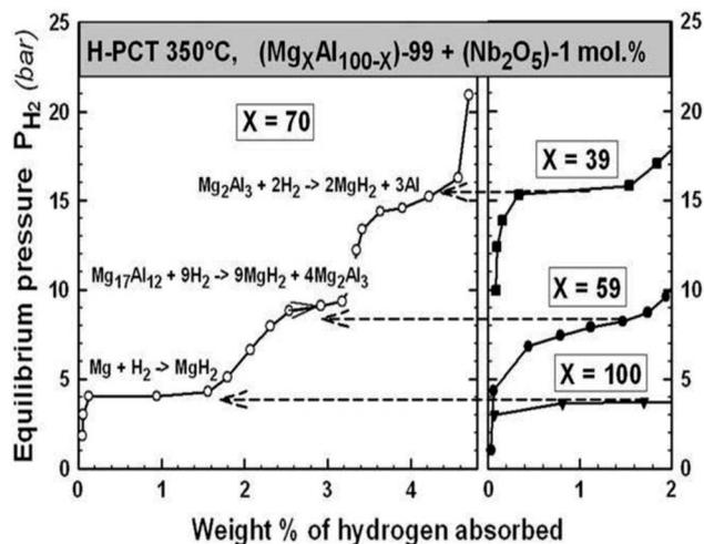
Fig. 23 Summary of the PCT absorption curves of the  $(\text{Mg}_x\text{Al}_{100-x})-99 + (\text{Nb}_2\text{O}_5) - 1$  mol.% samples. The 3 steps of transformation from the  $X = 70$  samples are compared to the absorption curves of the  $X = 100$  (Mg),  $X = 59$  ( $\text{Mg}_{17}\text{Al}_{12}$ ) and  $X = 39$  ( $\text{Mg}_2\text{Al}_3$ ) compounds.<sup>96</sup>
