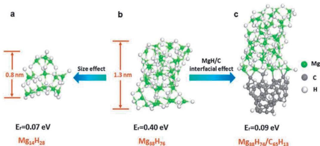
Fig. 18 Reaction energy ( $E_r$ ) for hydrogen release from clusters of pure  $\text{MgH}_2$  and  $\text{MgH}_2/\text{C}$ . (a)  $\text{Mg}_{14}\text{H}_{28}$  cluster, (b)  $\text{Mg}_{38}\text{H}_{76}$  cluster, and (c)  $\text{Mg}_{38}\text{H}_{74}$  adsorbed on a cluster of amorphous carbon.<sup>74</sup>
