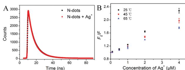
**Fig. 6** (A) Time-resolved fluorescence decay curves of the N-dot solution before and after the addition of 10  $\mu\text{M}$   $\text{Ag}^+$ . (B) Stern–Volmer plots at three different temperatures. (The concentration of the N-dot solution was 100  $\mu\text{g mL}^{-1}$ .)
