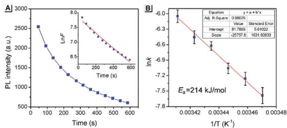
**Fig. 6** (A) The thermal fading kinetics of ground **SBA** at 20 °C. Inset: The curves fitted with first-order reaction dynamics. (B) The rate constants obtained from different temperatures fitted with Arrhenius expressions. The inset shows the fitting parameters.
