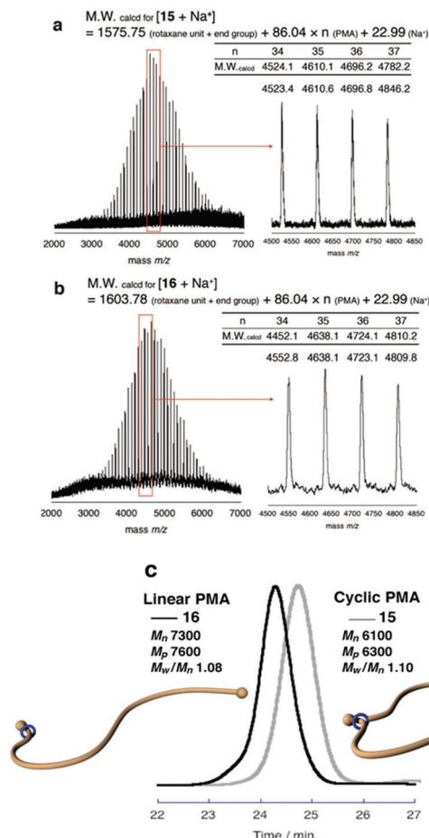
Fig. 3 MALDI-TOF mass spectra of macromolecular [1]rotaxane **15** (a) and macromolecular [2]rotaxane **16** (b). SEC traces (c) of **15** (Light gray line) and **16** (Black line) (eluent: CHCl<sub>3</sub>, 0.85 mL min<sup>-1</sup>, PSt standards).
