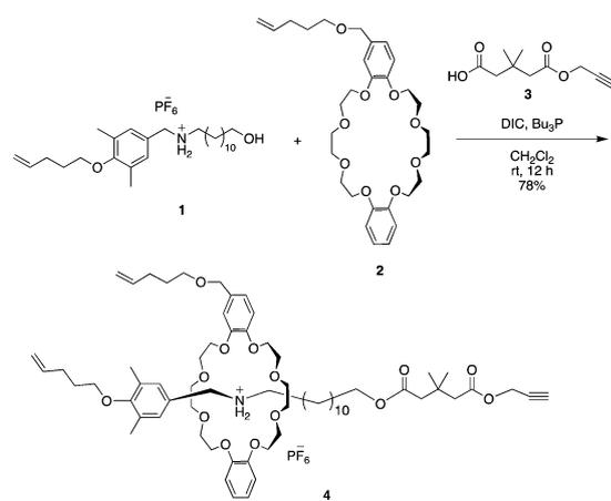
**Scheme 1** Synthesis of the temporarily stabilized rotaxane terminal unit **4**: ammonium salt **1** and crown ether **2** *in situ* generate a semi[2]rotaxane intermediate, the neopentyl group kinetically stabilizes rotaxane **4**.
