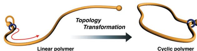
Fig. 1 Schematic illustration for polymer topological transformation from linear-to-cyclic utilizing the rotaxane protocol, which is facilitated by the positional change of the wheel from the initial to opposite end along the polymer chain.
