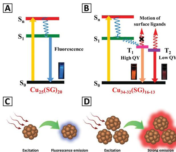
Fig. 1 Schematics of the energy levels and excitation/emission processes in (A) isolated  $\text{Cu}_{25}(\text{SG})_{20}$  NCs and (B) aggregated  $\text{Cu}_{34-32}(\text{SG})_{16-13}$  NCs. Adapted with permission from ref. 92, Copyright 2019, ACS. (C and D) Give a schematic representation of the emission from the isolated metal NCs and the aggregated clusters, respectively.
