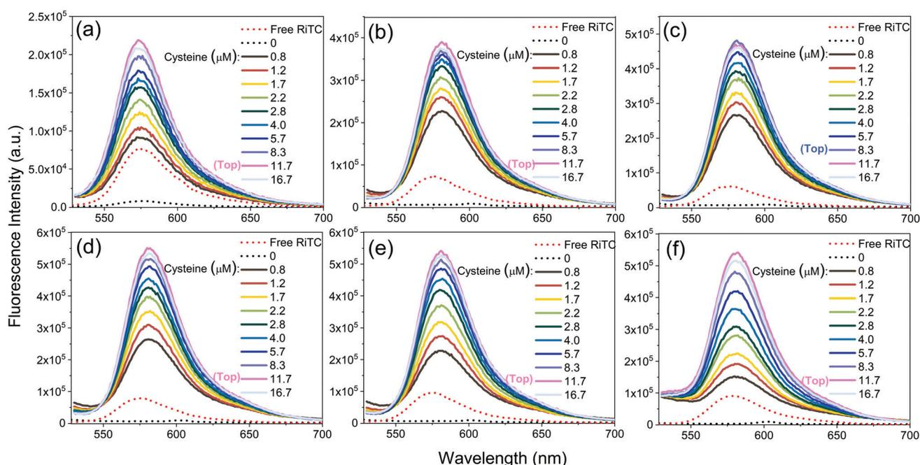
**Fig. 3** Fluorescence spectra of free RiTC and Au@Ag-RiTC NPs with different Ag shell thicknesses upon addition of different amounts of cysteine: 0 nm (a), 1.3 nm (b), 2.1 nm (c), 3.2 nm (d), 4.5 nm (e), and 5.6 nm (f); 0 nm refers to Au NPs.  $\lambda_{\text{EX}} = 520\text{ nm}$ .
