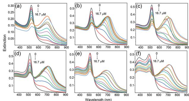
**Fig. 2** Extinction spectra of Au@Ag-RiTC NP solution with various Ag shell thicknesses upon gradual addition of cysteine: 0 nm (a), 1.3 nm (b), 2.1 nm (c), 3.2 nm (d), 4.5 nm (e), and 5.6 nm (f); 0 nm refers to Au NPs.
