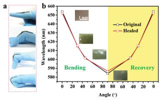
Fig. 6 Strain-induced color shifting properties of the red-colored  $SiO_2/PEG-UPy50$  PE for different bending angles. (a) Illustration of the bending angle of the elastomer and the corresponding reflectance peak position (b) of the original and self-healed SiO<sub>2</sub>/PEG-UPy50 PE. Inset in (b): photographs of the original SiO<sub>2</sub>/PEG-UPy50 PE for the different bending angles.
