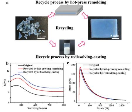
Fig. 5 (a) Recycling properties of the PEs through the hot-press molding and the redissolving-casting processes. Reflectance spectra (b) and stressstrain curves (c) of the original SiO<sub>2</sub>/PEG-UPy50 PE and the corresponding recycled samples by redissolving-casting and hot-press remolding.
