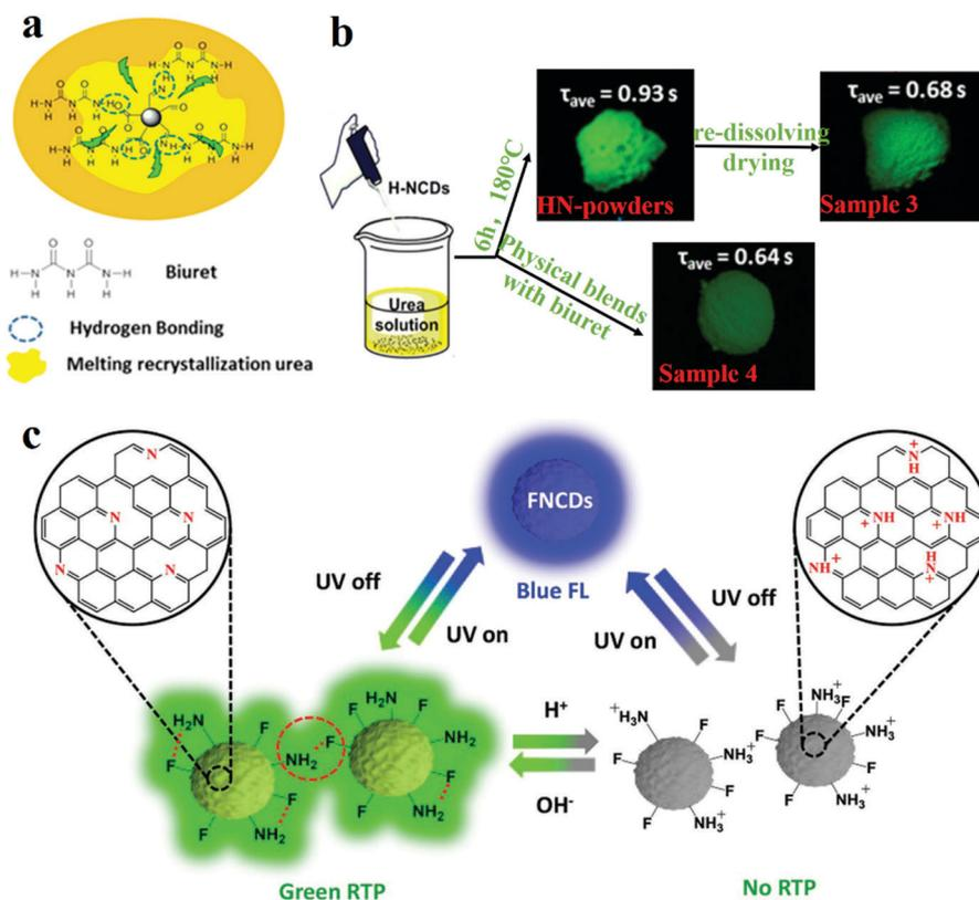
**Fig. 5** Schematic of the RTP mechanism and the factors influencing matrix and matrix-free CDs. (a) RTP model of NCDs. (b) Experiments for verification of the influence of hydrogen bonding on phosphorescence lifetime. Reprinted with permission from ref. 135, Copyright 2016, American Chemical Society. (c) Mechanism proposed by Long *et al.* for the pH response of RTP in FNCDs. Reprinted with permission from ref. 130, Copyright 2018, Wiley-VCH Verlag GmbH & Co. KGaA.
