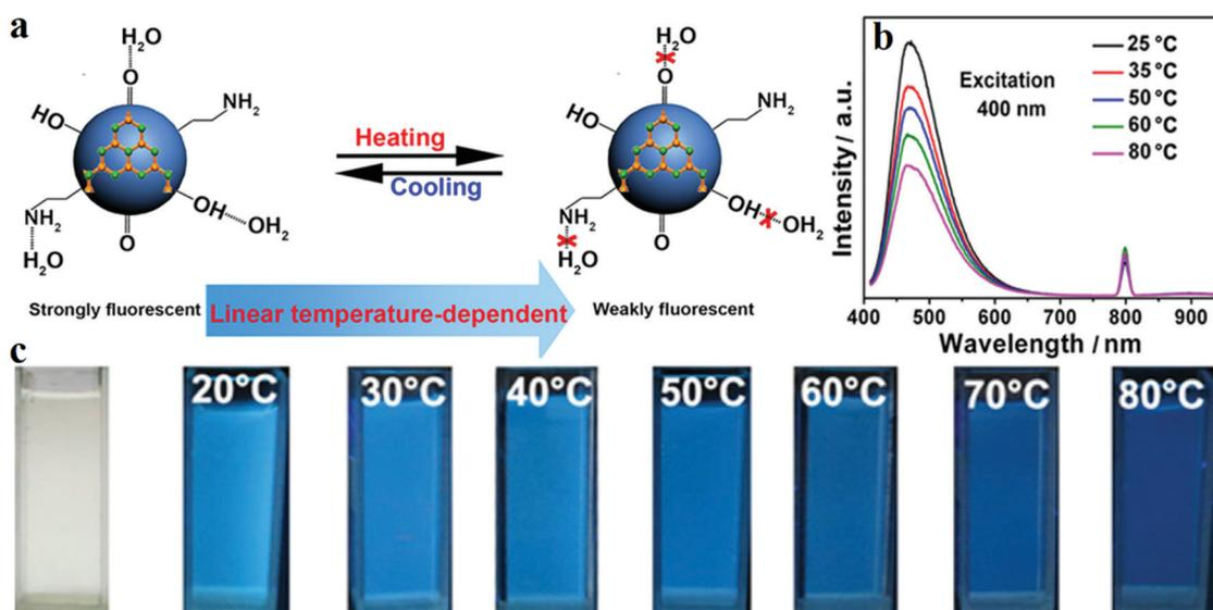
**Fig. 11** (a) Schematic diagram of a N-CD temperature sensor. (b) Fluorescence intensity decreases with increasing temperature. (c) Images of the N-CD sensor under UV illumination at different temperatures. Reprinted with permission from ref. 156, Copyright 2015, American Chemical Society.
