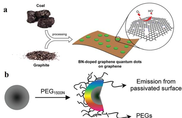
**Fig. 3** Schematic representations of the heteroatom doping and surface passivation approaches of CD functionalisation, reprinted with permission from ref. (a) Illustration of the preparation procedure for the BN-GQD/graphene nanocomposite, reprinted with permission from ref. 93, Copyright 2014, American Chemical Society. (b) Functionalisation of CD surfaces with PEG, reprinted with permission from ref. 14, Copyright 2006, American Chemical Society.
