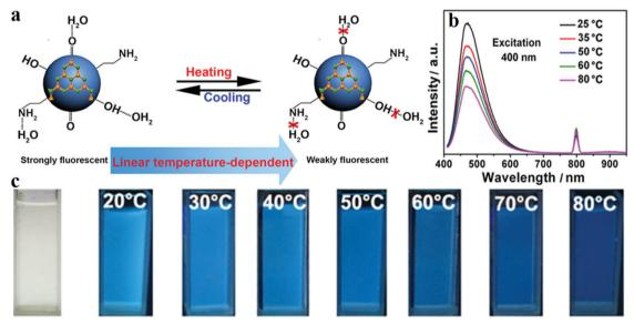
Fig. 11 (a) Schematic diagram of a N-CD temperature sensor. (b) Fluorescence intensity decreases with increasing temperature. (c) Images of the N-CD sensor under UV illumination at different temperatures. Reprinted with permission from ref. 156, Copyright 2015, American Chemical Society.
