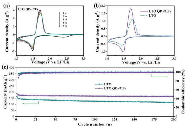
Fig. 5 (a) Five CV curves of LTO QDs/CFs at 1 mV s<sup>-1</sup>, (b) comparison of CV curves between LTO and LTO QDs/CFs at 0.5 mV s<sup>-1</sup>, and (c) cycling performance at 1C (1C = 175 mA g<sup>-1</sup>).
