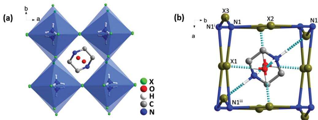
Fig. 1 (a) The crystal structure of  $[(C_4N_2H_{12})(NH_4X_3) \cdot H_2O]$ . (b) Hydrogen bond diagrams of the simplified perovskite frameworks viewed along the  $c$  axis ( $X = Br, Cl, I$ ). Symmetry codes: (i)  $X, 0.5 - Y, -Z$ ; (ii)  $-X, 0.5 + Y, 0.5 - Z$ ; (iii)  $-X, -Y, 0.5 + Z$ .
