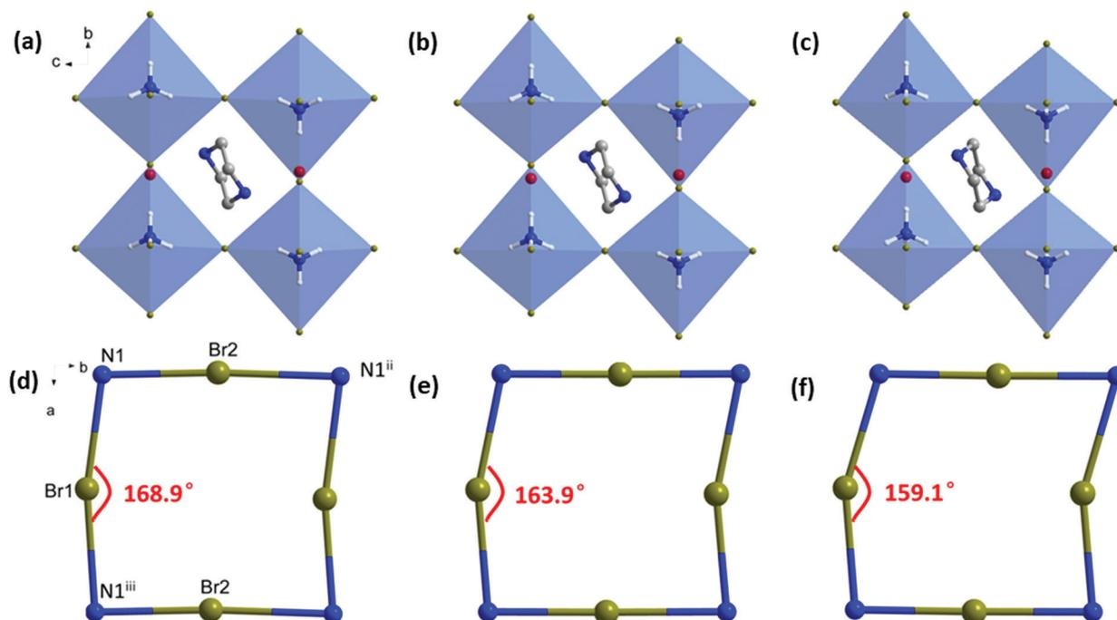
Fig. 5 The packing diagrams of **PIP-Br** at pressures of 0 GPa (a), 1.99 GPa (b) and 4.86 GPa (c). (d)–(f) are the revolution plots of the N1–Br1–N1<sup>iii</sup> angle at 0 GPa, 1.99 GPa and 4.86 GPa, respectively. Symmetry codes: (ii)  $-X, 0.5 + Y, 0.5 - Z$ ; (iii)  $-X, -Y, 0.5 + Z$ .
