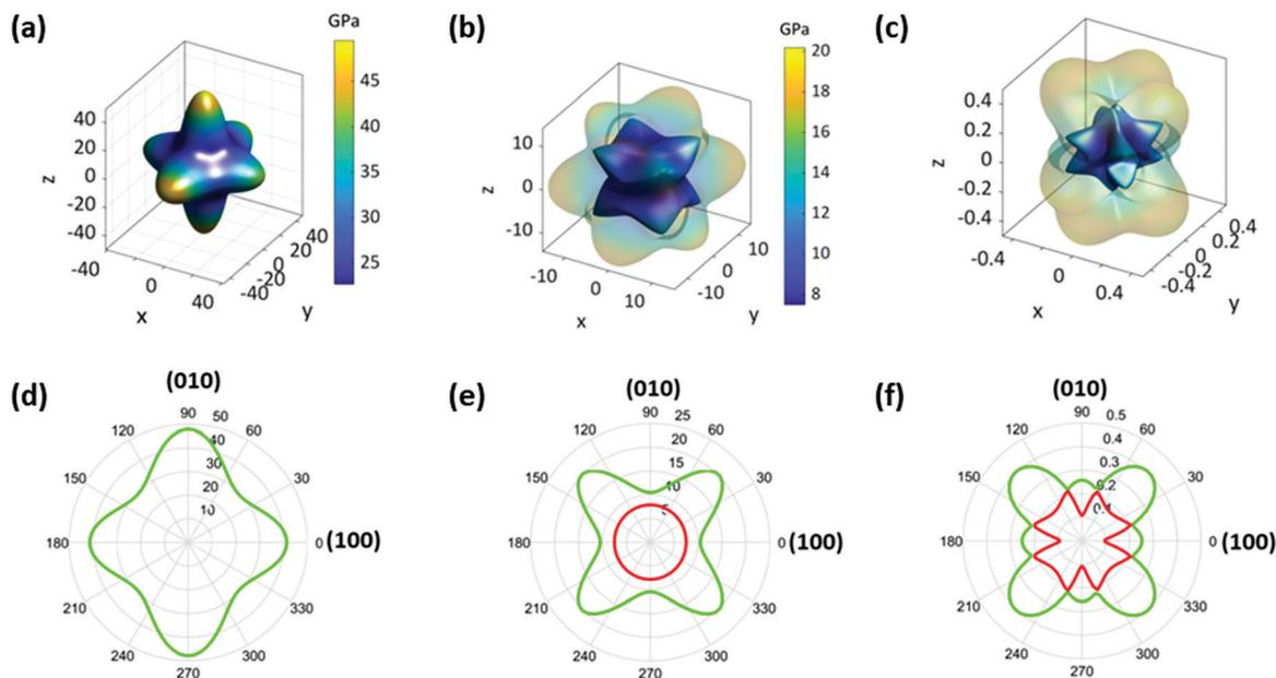
**Fig. 3** The 3D and 2D representations of Young's modulus (a) and (d), shear modulus (b) and (e) and Poisson's ratio (c) and (f) for **PIP-Br**. In (b) and (c), the transparent outer layer and non-transparent inner layers represent the maximum and minimum values, respectively. In (e) and (f), the green outer line and red inner line represent the maximum and minimum values, respectively.
