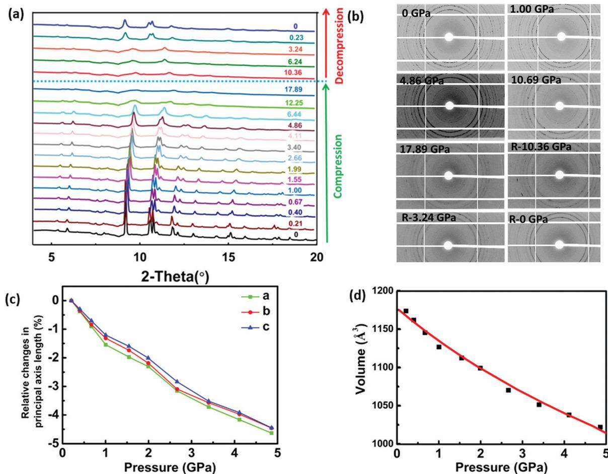
Fig. 4 The HP-XRD data for **PIP-Br**: (a) *in situ* HP-XRD patterns during compression and decompression (pressure unit is GPa). (b) Representative 2D images at selected pressures. 'R-' means decompression process. (c) Pressure-dependent relative changes in length for the three principal axes. (d) The evolution of cell unit volume as a function of pressure. The red solid line represents the second-order Birch–Murnaghan fit to the experimental data.
