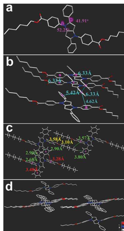
Fig. 7 The crystal structure (a), intermolecular interactions (b and c), and packing patterns (d) of **TPPP-C6**. Green and red lines represent the inter- and intramolecular C-H $\cdots$  $\pi$  interactions, respectively, and yellow lines represent the C-H $\cdots$ O interactions in Fig. 8(c).
