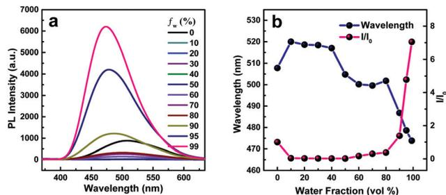
Fig. 2 (a) Fluorescence spectra of TPPP-C6 in THF/water mixtures with different water fractions ( $f_w$ : 0–99%); (b) plot of the wavelength and the ratio of the maximum fluorescence intensity of TPPP-C6 vs. the water fraction,  $I_0$  = emission intensity in pure THF solution. Excitation wavelength: 322 nm, concentration:  $1 \times 10^{-5}$  M.
