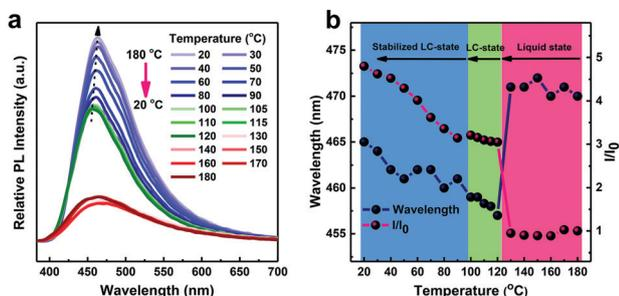
Fig. 6 Temperature-dependent fluorescence spectra (a) and plot of wavelength and fluorescence intensity vs. temperature of **TPPP-C6** (b) during the cooling process from  $180^\circ\text{C}$  to room temperature under  $360 \text{ nm}$  UV light.
