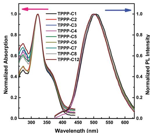
Fig. 1 Normalized UV-vis absorption (left) and fluorescence (right) spectra of TPPP derivatives in THF solution. Concentration:  $1 \times 10^{-5}$  M, excitation wavelength: 322 nm.
