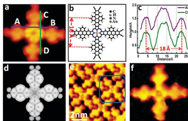
**Fig. 2** STM images and models of the cross-like structure at the sub-molecular level. (a) HR-STM image ( $V_s = -0.90$  V and  $I_s = -0.08$  nA). (b) Molecular model. (c) Height profiles along the lines indicated in Fig. 2a. (d) Simulated STM image. (e) STM image recorded by functionalizing the STM tip *via* empirical adsorption of an Au adatom ( $V_s = -0.83$  V and  $I_s = -0.10$  nA). (f) Detailed STM image for a single Au-Pc compound.
