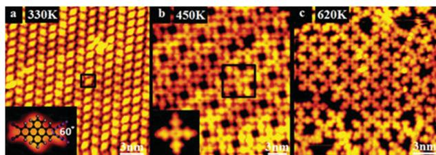
**Fig. 1** STM images of DTTCN molecules adsorbed on an Au(111) surface that experience a hierarchical on-surface reaction driven by thermal treatments. (a) The assembly structure; the inset presents the structural model and high-resolution STM (HR-STM) image for a single DTTCN molecule ( $V_s = -2.8$  V and  $I_s = -0.04$  nA). (b) The cross-like supramolecular network ( $V_s = -1.80$  V and  $I_s = -0.03$  nA). (c) The mesh-like network ( $V_s = -1.10$  V and  $I_s = -0.03$  nA).
