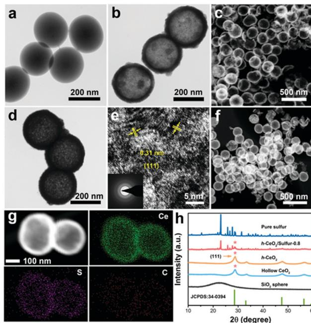
Fig. 2 TEM images of (a) SiO<sub>2</sub> and (b) hollow CeO<sub>2</sub>. (c) SEM image of hollow CeO<sub>2</sub>. (d) TEM image and (e) HRTEM image of h-CeO<sub>2</sub> (the inset shows a SAED pattern). (f) HAADF-TEM image and (g) EDS elemental mapping of h-CeO<sub>2</sub>/sulfur-0.8. (h) XRD patterns.
