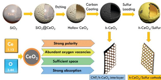
Fig. 1 Illustration of synthetic procedures of a h-CeO<sub>2</sub>/sulfur cathode and a CNT/h-CeO<sub>2</sub> interlayer for Li-S batteries.
