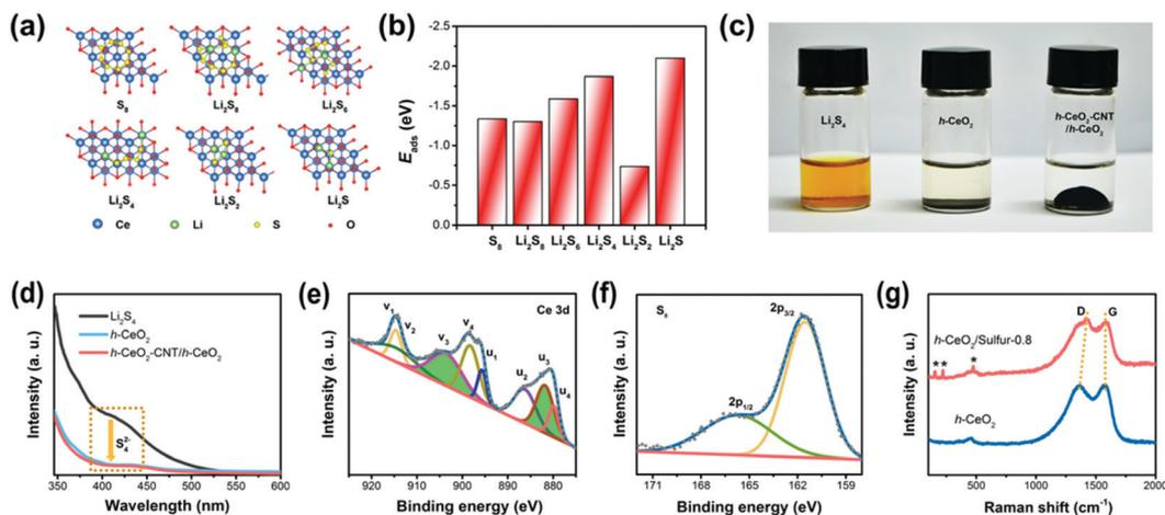
**Fig. 3** (a) Optimized geometries and (b) adsorption energies of  $S_8$  and polysulfides on ceria surfaces; (c) digital photographs showing the adsorption ability of  $Li_2S_4$  after 12 h; (d) UV/vis absorption spectra of lithium polysulfide ( $Li_2S_4$ /DME) solution before and after adding  $h-CeO_2$  and  $h-CeO_2$ -CNT/ $h-CeO_2$  interlayers; (e) and (f) high-resolution XPS spectra of  $h-CeO_2$ /sulfur-0.8; and (g) Raman spectra of  $h-CeO_2$  and  $h-CeO_2$ /sulfur-0.8.
