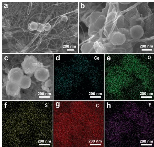
Fig. 5 (a) Initial CNT/h-CeO<sub>2</sub> interlayer; (b) CNT/h-CeO<sub>2</sub> interlayer after 500 cycles; and (c–h) the images of SEM and EDX elemental mapping.
