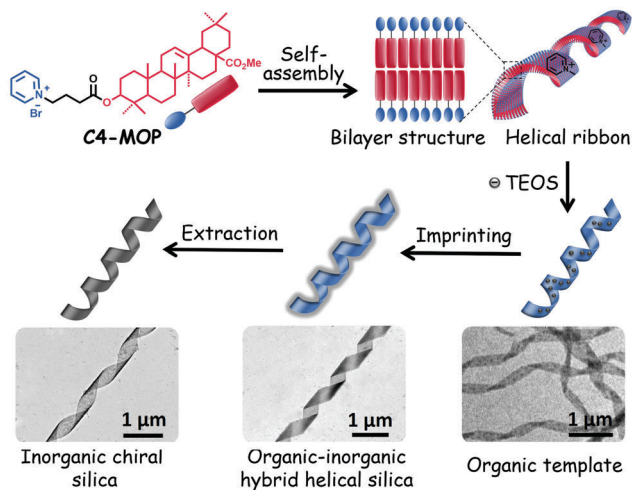
Scheme 1 Schematic of the fabrication of helical ribbons assembled from C4-MOP and its chirality imprinting to inorganic silica.
