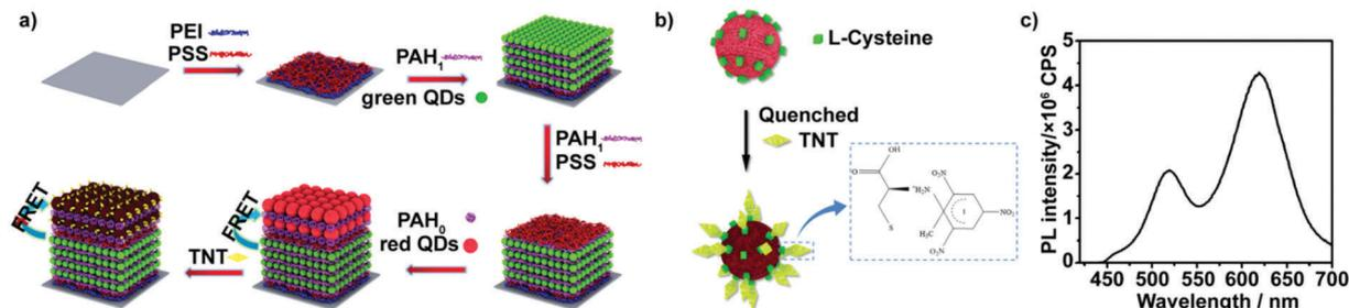
Fig. 1 (a) Scheme for fabrication of QD multilayers-coated film for visual determination of TNT and the detection mechanism. (b) Schematic illustrations for the quenching mechanism of fluorescence by TNT analyte. (c) Fluorescence spectra of (PEI/PSS)<sub>3</sub>(PAH/green QDs)<sub>10</sub>(PAH/PSS)<sub>3</sub>(PAH/red QDs)<sub>5</sub> multilayers deposited on glass substrates.
