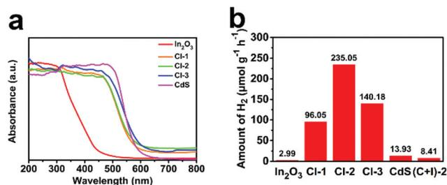
**Fig. 5** (a) UV-vis DRS of  $\text{In}_2\text{O}_3$ , CdS and CdS/ $\text{In}_2\text{O}_3$  heterostructures; (b) photocatalytic activities of different samples towards visible-light hydrogen production from water.
