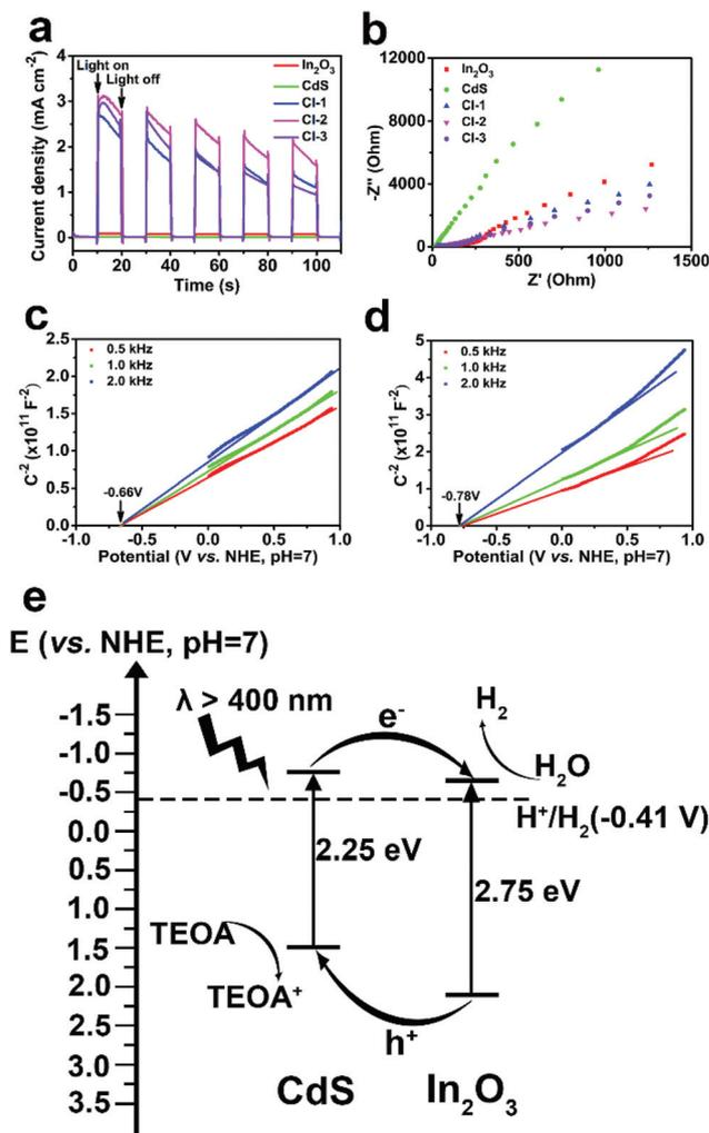
Fig. 7 (a) Transient photocurrent responses and (b) EIS Nyquist plots of  $\text{In}_2\text{O}_3$ ,  $\text{CdS}$  and  $\text{CdS}/\text{In}_2\text{O}_3$  heterostructures; Mott-Schottky plots of (c)  $\text{In}_2\text{O}_3$  nanotubes and (d)  $\text{CdS}$  nanoparticles; (e) schematic diagram of the band structure of  $\text{CdS}/\text{In}_2\text{O}_3$  heterostructure.
