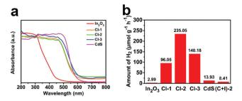
Fig. 5 (a) UV-vis DRS of In<sub>2</sub>O<sub>3</sub>, CdS and CdS/In<sub>2</sub>O<sub>3</sub> heterostructures; (b) photocatalytic activities of different samples towards visible-light hydrogen production from water.
