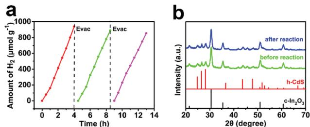
**Fig. 8** (a) Photocatalytic stability of CdS/In<sub>2</sub>O<sub>3</sub>-2 towards visible-light hydrogen production; (b) XRD patterns of CdS/In<sub>2</sub>O<sub>3</sub>-2 before and after the photocatalytic cyclic test.
