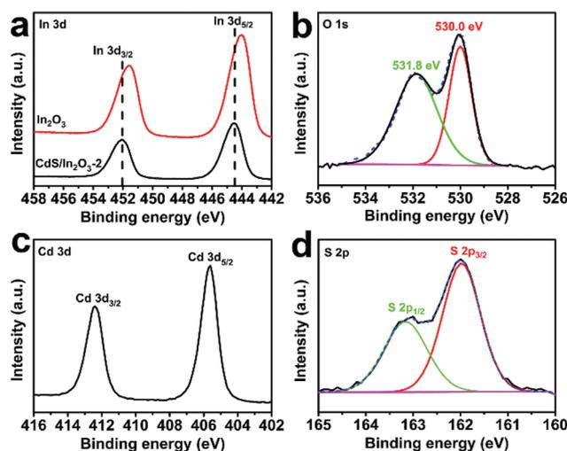
**Fig. 4** High resolution XPS spectra of (a) In 3d, (b) O 1s, (c) Cd 3d and (d) S 2p in CdS/In<sub>2</sub>O<sub>3</sub>-2. The red curve in (a) is the high resolution XPS spectrum of In 3d in In<sub>2</sub>O<sub>3</sub> nanotubes.
