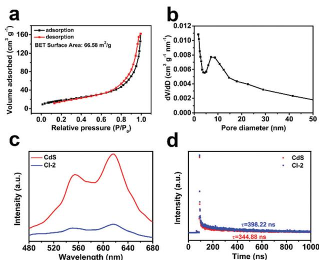
**Fig. 6** (a) Nitrogen adsorption-desorption isotherm and (b) pore size distribution of CdS/ $\text{In}_2\text{O}_3$ -2; (c) steady-state PL spectra and (d) PL decay spectra of CdS and CdS/ $\text{In}_2\text{O}_3$ -2.
