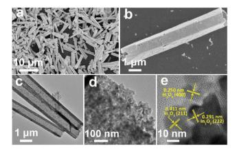
Fig. 2 (a, b) SEM, (c, d) TEM and (e) HRTEM images of In<sub>2</sub>O<sub>3</sub> nanotubes.
