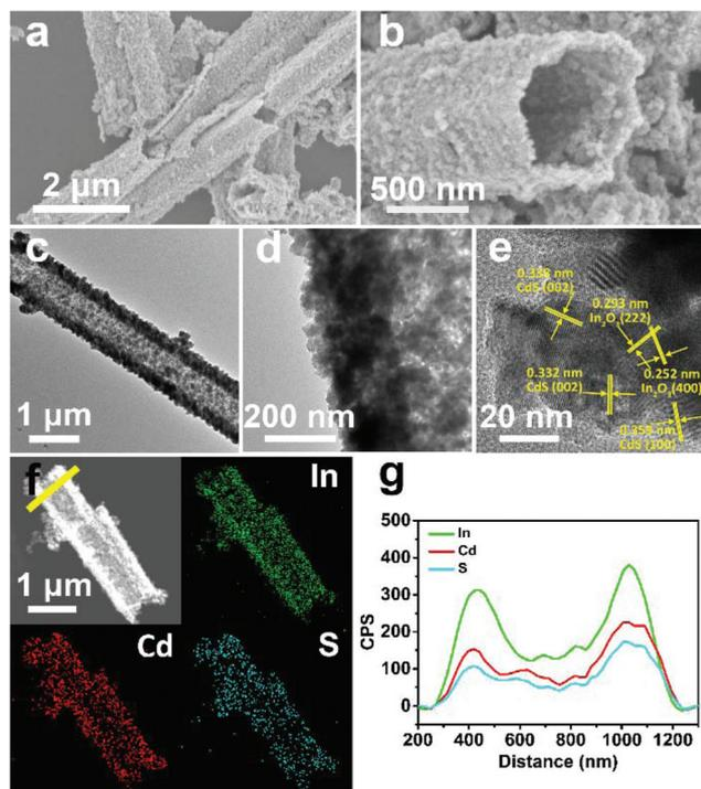
**Fig. 3** (a, b) SEM, (c, d) TEM, (e) HRTEM and (f) HAADF-STEM and EDS mapping images of CdS/In<sub>2</sub>O<sub>3</sub>-2; (g) EDS line scan profiles of CdS/In<sub>2</sub>O<sub>3</sub>-2 obtained along the yellow line in (f).
