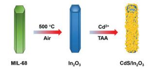
Scheme 1 Schematic of the synthesis process of CdS/In<sub>2</sub>O<sub>3</sub> hierarchical nanotubes.
