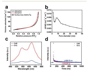
Fig. 6 (a) Nitrogen adsorption-desorption isotherm and (b) pore size distribution of CdS/In<sub>2</sub>O<sub>3</sub>-2; (c) steady-state PL spectra and (d) PL decay spectra of CdS and CdS/In<sub>2</sub>O<sub>3</sub>-2.
