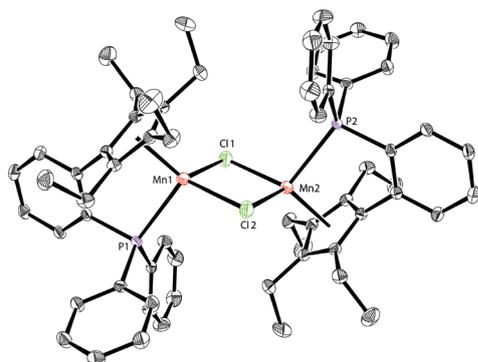
**Fig. 2** Molecular structure of **1a** with thermal ellipsoids at 30% probability. H atoms are omitted for clarity. Selected bond lengths [Å] and angles [°]:  $\text{Mn}(1)\text{-Cl}(1)$ : 2.3909(7),  $\text{Mn}(1)\text{-Cl}(2)$ : 2.4603(7),  $\text{Mn}(1)\text{-P}(1)$ : 2.6066(6), and  $\text{Cl}(1)\text{-Mn}(1)\text{-Cl}(2)$ : 94.71(3).
