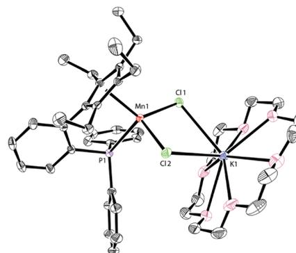
**Fig. 3** Molecular structure of **2** with thermal ellipsoids at 30% probability. H atoms are omitted for clarity. Selected bond lengths [Å] and angles [°]: Mn(1)–Cl(1): 2.3997(6), Mn(1)–Cl(2): 2.3844(7), Mn(1)–P(1): 2.7264(6), K(1)–Cl(1): 3.1928(8), K(1)–Cl(2): 3.2865(8), Cl(1)–Mn(1)–Cl(2): 99.83(2), and Cl(1)–K(1)–Cl(2): 65.879(16).
