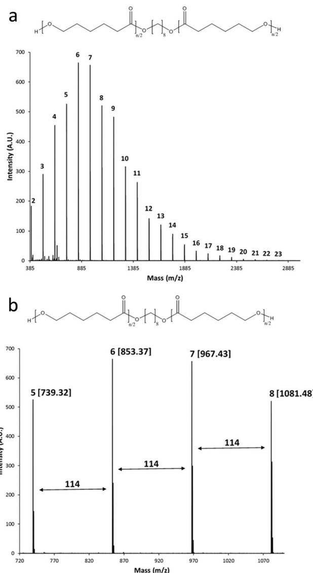
**Fig. 2** (a) MALDI TOF mass spectrum of the HOPCLOH ( $M_n(\text{NMR}) = 645$ , Table 1, first line), the number indicates the degree of polymerization (DP) of each peak, and (b) expanded view for the 5–8 CL repeating units, in brackets the mass with sodium doped, 114 is the molecular weight of the CL monomer.
