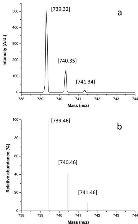
Fig. 3 MALDI-TOF mass spectrum view for the 738–744 *m/z* fragments of the HOPCLOH (Fig. 2b), degree of polymerization (DP) = 5 [OctPCL<sub>5</sub>, HO(CH<sub>2</sub>)<sub>8</sub>O[CO(CH<sub>2</sub>)<sub>5</sub>O]<sub>5</sub>H Na<sup>+</sup>], (a) experimental spectrum, and (b) isotopic distribution calculated for DP = 5 [C<sub>38</sub>O<sub>12</sub>H<sub>68</sub>Na<sup>+</sup>, in <http://www.chemcalc.org>].<sup>25</sup> The mass with doped sodium is given in brackets.
