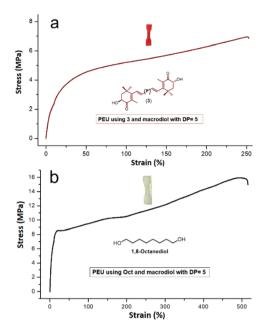
Fig. 7 Representative tensile data for PEUs derived from compound 3 (a) and those derived from 1,8-octanediol (Oct) (b).
