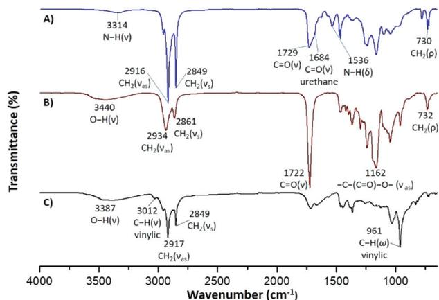
Fig. 5 FTIR spectra of (A) PEUs synthesized from a macrodiol with DP = 5 and **1** as chain extender, (B) macrodiol with DP = 5, and (C) compound **1**.
