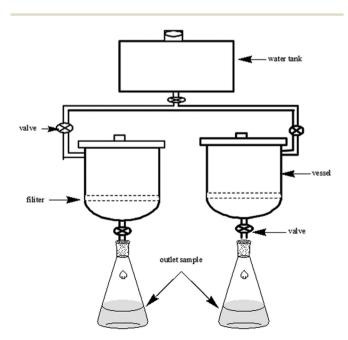
Fig. 14 Experimental device setup for a fertilizer release study. 40
