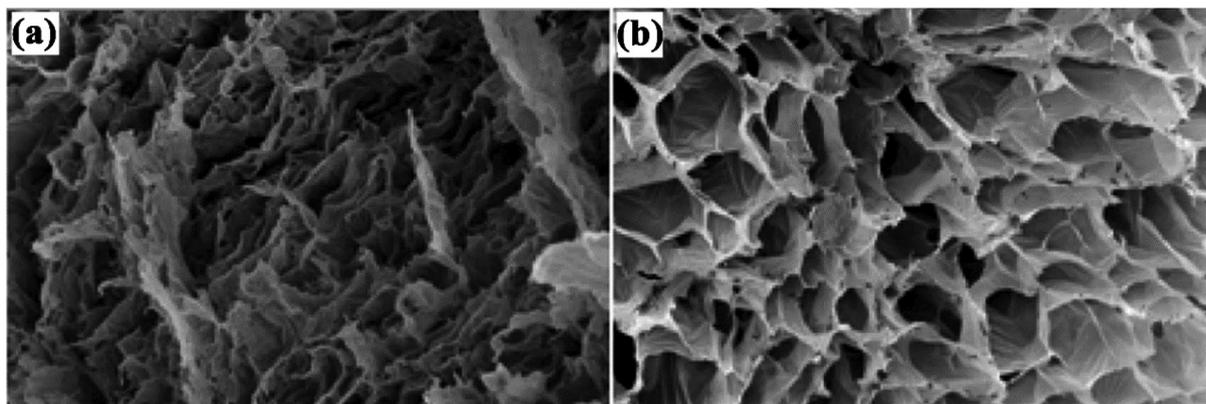
Fig. 3 SEM images of (a) hydrolyzed hydrogel (1 : 1) and (b) hydrolyzed hydrogel (3 : 1).<sup>58</sup> Reprinted with permission from ref. 58. Copyright (2013) American Chemical Society.
