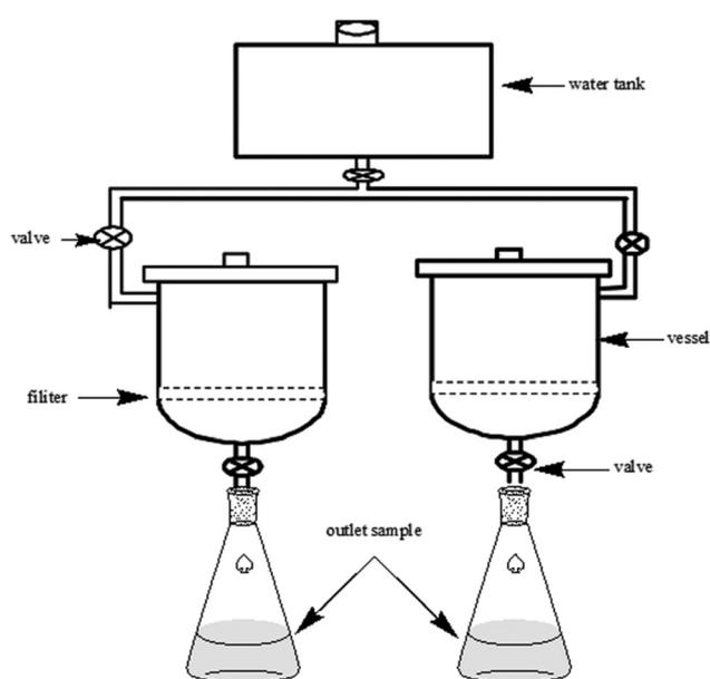
Fig. 14 Experimental device setup for a fertilizer release study.<sup>40</sup>
