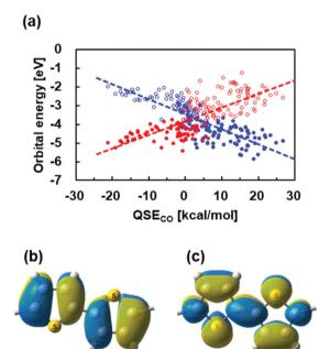
Fig. 7 (a) Plots of HOCO (filled) and LUCO (empty) energy levels against QSE<sub>CO</sub> of the 179 copolymers. Blue and red symbols indicate aromatic and quinoidal orbitals, respectively. (b) The aromatic type orbital (HOCO) and (c) quinoid type orbital (LUCO) of poly(thiophene).
