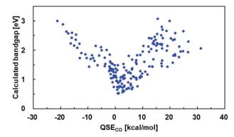
Fig. 4 Correlation between QSE<sub>CO</sub> and a bandgap of the 179 alternate copolymers.
