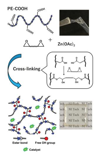
Fig. 1 Schematic of the present molecular design. Free OH groups are generated by the epoxy-opening reaction with COOH groups in PE-COOH during the cross-linking reaction. The pictures of samples before and after cross-linking are also shown.
