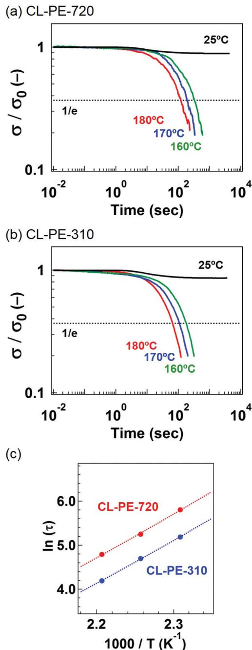
**Fig. 4** Stress-relaxation spectra for (a) CL-PE-720 and (b) CL-PE-310, where the stress ( $\sigma$ ) is normalized by the initial stress ( $\sigma_0$ ). The dotted lines in (a) and (b) indicate the point at  $\sigma/\sigma_0 = 1/e (=0.3679)$ . (c) Arrhenius plots of  $\tau$  as a function of inverse temperatures.
