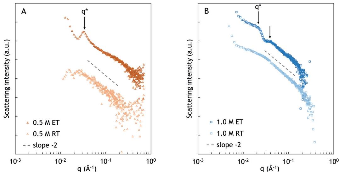
**Fig. 4** SAXS spectra of PNIPAM-*b*-PDMAEMA and PNIPAM-*b*-PAA-*b*-PNIPAM in 0.5 M (A) and 1.0 M (B) NaCl at 27 °C (RT) and 67 °C (ET). As a guide to the eye, a dashed line is displayed to indicate a slope of  $-2$ . The presented data were corrected for solvent contributions and plotted on a log–log scale. Scattering intensities of the ET data were adjusted for clear display.
