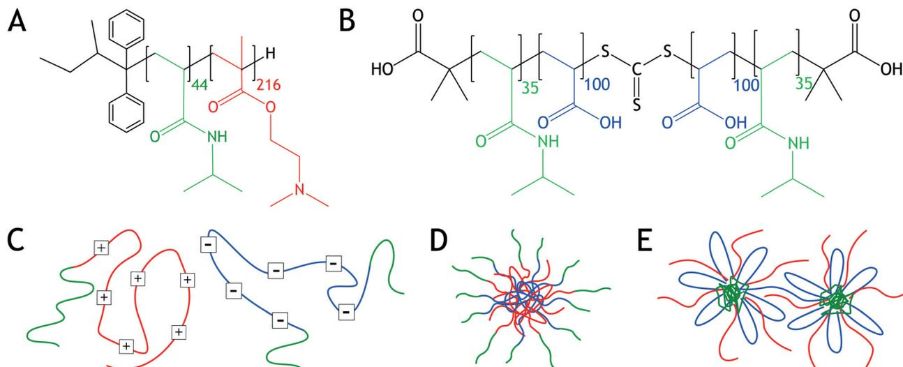
**Fig. 1** Chemical structures of (a) cationic PNIPAM-*b*-PDMAEMA, which was synthesized by anionic polymerization, and (b) PNIPAM-*b*-PAA-*b*-PNIPAM, which was synthesized by reversible addition fragmentation chain transfer (RAFT) polymerization. Schematic representations of (c) PNIPAM-*b*-PDMAEMA and PNIPAM-*b*-PAA-*b*-PNIPAM, (d) a C3M, and (e) PCMs. The red block represents PDMAEMA, the blue block PAA and the green blocks PNIPAM.
