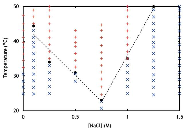
**Fig. 2** Light scattering was used to determine the  $T_{cp}$  of samples containing PNIPAM-*b*-PDMAEMA and PNIPAM-*b*-PAA-*b*-PNIPAM with varying concentrations of NaCl. The results were used to create a phase diagram; the blue crosses represent a one phase system, and the red pluses represent an aggregated system. The dotted lines represent the phase boundary that was deduced from the observed  $T_{cp}$ s (black dots).
