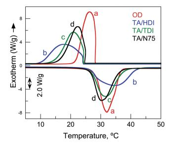
**Fig. 6** Thermal behavior (DSC) from the first cooling and the second heating of: (a) OD; (b) TA/HDI; (c) TA/TDI; (d) TA/N75.
