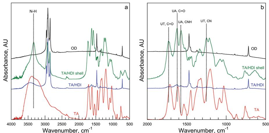
Fig. 4 FTIR spectra from OD, TA, and TA/HDI (both the OD-filled PH and the PUU shell): (a) spectra from 500 to 4000  $\text{cm}^{-1}$ ; (b) spectra from 500 to 2000  $\text{cm}^{-1}$  showing the main urethane and urea bands.
