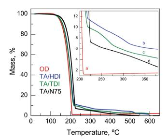
**Fig. 5** Thermal decomposition in air (TGA) of: (a) OD; (b) TA/HDI; (c) TA/TDI; (d) TA/N75. Inset: enlargement of the results at low residual masses.
