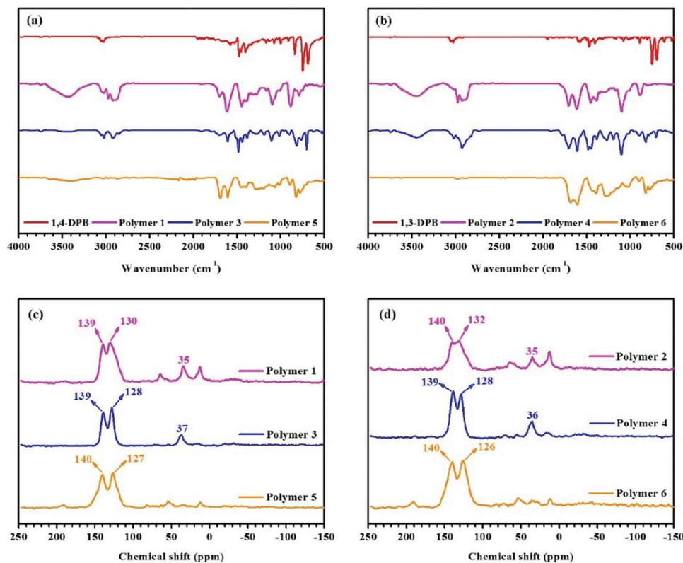
Fig. 1 FT-IR spectrum of (a) 1,4-DPB and 1,4-DPB-based polymer materials, and (b) 1,3-DPB and 1,3-DPB-based polymer materials; solid state cross-polarization (CP)  $^{13}\text{C}$  MAS natural abundance NMR spectrum of (c) 1,4-DPB-based polymer materials, and (d) 1,3-DPB-based polymer materials.
