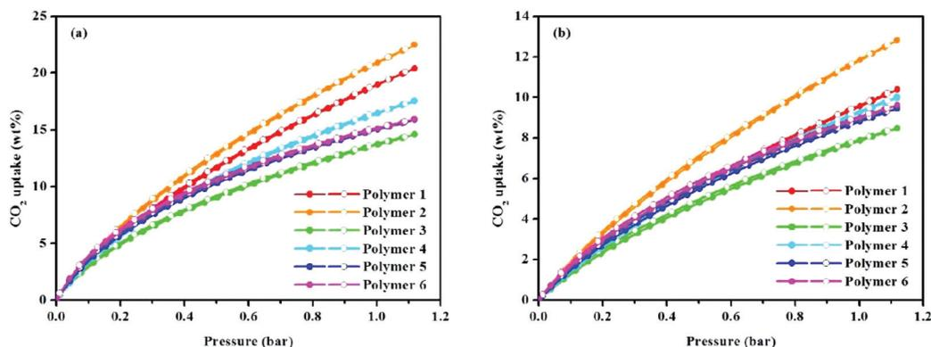
Fig. 4 (a) Volumetric CO<sub>2</sub> adsorption and desorption isotherms up to 1.13 bar at 273.15 K, and (b) volumetric CO<sub>2</sub> adsorption and desorption isotherms up to 1.13 bar at 298.15 K.
