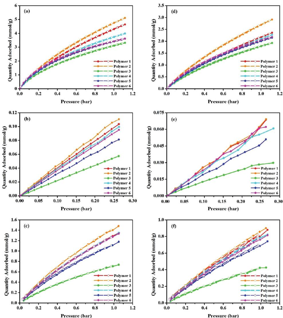
Fig. 5 Adsorption isotherms of CO<sub>2</sub> (a), N<sub>2</sub> (b), CH<sub>4</sub> (c) gases at 273.15 K, and CO<sub>2</sub> (d), N<sub>2</sub> (e), CH<sub>4</sub> (f) gases at 298.15 K for polymer 1 to polymer 6. Filled symbols represent adsorption and open symbols represent desorption.
