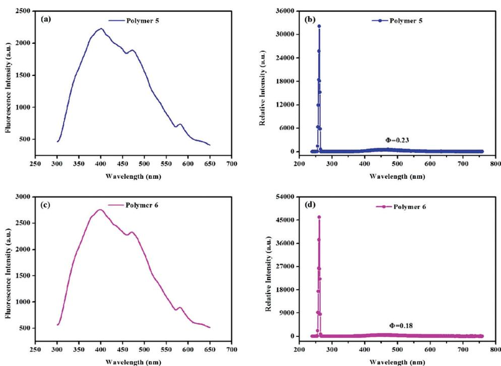
Fig. 6 Solid state fluorescence excitation spectrum of polymer 5 (a,  $\lambda_{\text{em}} = 280$  nm,  $\lambda_{\text{ex}} = 466$  nm), the absolute solid state fluorescence quantum yield of polymer 5 (b,  $\Phi = 0.23$ ), the solid state fluorescence excitation spectrum of polymer 6 (c,  $\lambda_{\text{em}} = 280$  nm,  $\lambda_{\text{ex}} = 466$  nm), and the absolute solid state fluorescence quantum yield of polymer 6 (d,  $\Phi = 0.18$ ).
