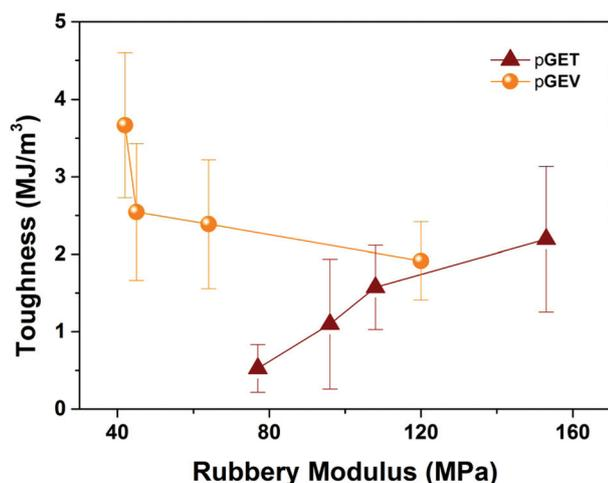
Fig. 6 Toughness *versus* rubbery modulus for the pGET and pGEV terpolymer formulations.
