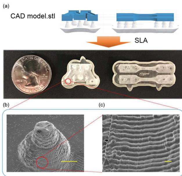
**Fig. 7** SLA printed object examples from the GEV 60–20–20 photore-sin with 2% TPO photoinitiator. (a) A printed “M” logo and dogbone tensile bars on the substrate. (b) Scanning electron microscopy image of a support cone was taken to observe the print resolution of objects, exhibiting the stair-casing feature. Scale bar is 100  $\mu\text{m}$ . (c) Magnified image with scale bar of 100  $\mu\text{m}$ .
