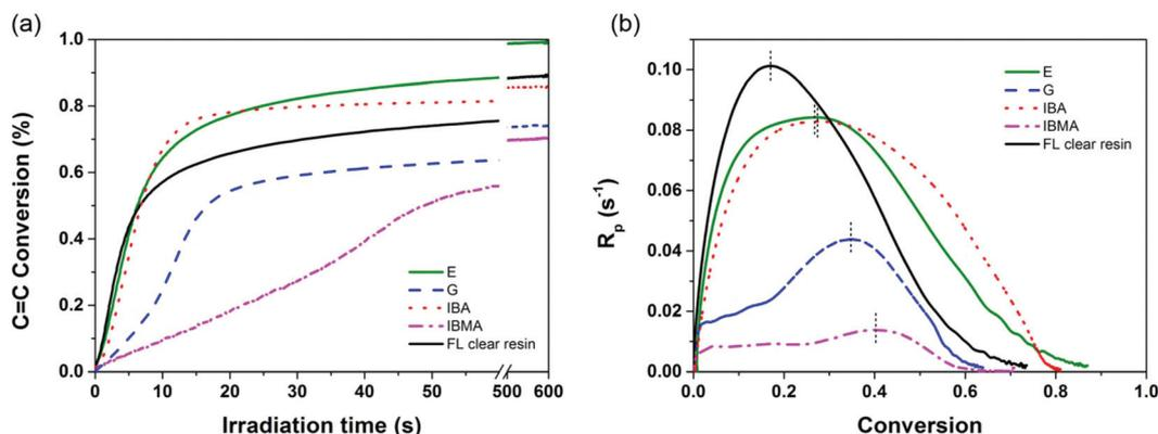
Fig. 2 Photopolymerization kinetic profiles of E and G compared to commercially available monomers (IBA and IBMA) and 3D printable prototype resins determined by real time-FTIR. (a) Plot of the double bond conversion as a function of UV irradiation time. (b) Plot of the polymerization rate as a function of monomer conversion at irradiation intensity of  $2 \text{ mW cm}^{-2}$ . The UV irradiation condition was  $365 \text{ nm}$  at  $2 \text{ mW cm}^{-2}$ .
