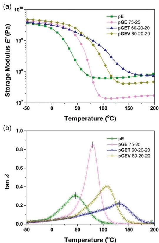
Fig. 4 Dynamic mechanical behavior of the formulated resins: (a) storage modulus and (b)  $\tan \delta$  of the photocured E polymer, binary pGE 75–25, and ternary pGET 60–20–20 and pGEV 60–20–20.
