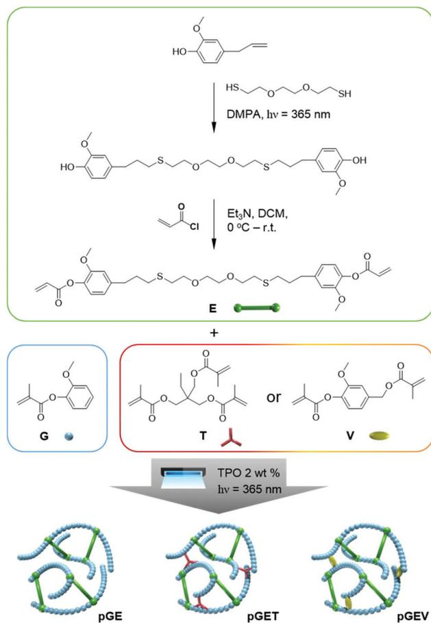
**Fig. 1** The synthetic route of the E monomer and its binary formulation GE, ternary formulations GET and GEV that are viable for photopolymerization with 2 wt% of TPO to form different cross-linking networks.
