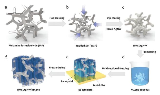
Fig. 1 Schematic illustrating the fabrication process of the BMF/AqNW/MXene hybrid sponge by a combination of mechanical hot-pressing (a→b), dip-coating (b $\rightarrow$ c), immersing (c $\rightarrow$ d), unidirectional freezing (d $\rightarrow$ e), and freeze-drying (e $\rightarrow$ f).
