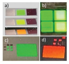
Fig. 7 Photographs of nanostructured samples, showing diffraction of white light of (a) an embedded grating (central square written at 1 mm s<sup>-1</sup>) observed at 3 different angles; (b) four surface gratings (written at 90, 100, 120, 150 mm  $s^{-1}$ ). Frames (c) and (d) show the same hybrid grating (large square, see also Fig. 9), observed from two different directions, rotated by 90°.
