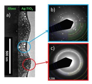
**Fig. 5** Locally dependent nanoparticle growth and matrix crystallization in SG structures: (a) HAADF-STEM image of film cross-section cut perpendicular to LIPSS for a structure written at 100 mm s $^{-1}$ . (b $^{-1}$ c) Diffraction patterns of the blue and red encircled zones in the HAADF-STEM image.
