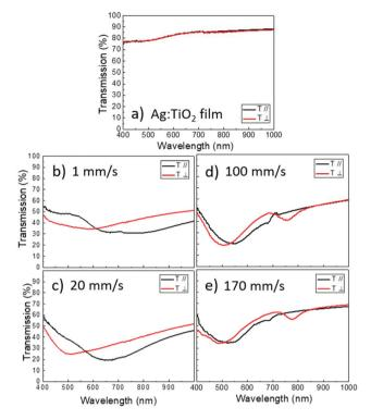
Fig. 6 Spectral response of the nanostructures. Transmission (T) spectra taken at 6° incidence angle for (a) the initial Ag:TiO $_2$  nanocomposite films before laser irradiation and different scan speeds of (b) 1 mm s $^{-1}$ , (c) 20 mm s $^{-1}$ , (d) 100 mm s $^{-1}$ , and (e) 170 mm s $^{-1}$ .  $\bot$  and  $\|$  refers to the probe polarization, respective to the laser polarization. Reflectance (R) and loss spectra (including absorption and scattering) are shown in the ESI.†
