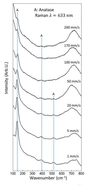
Fig. 4 Influence of the scan speed on the phase of the TiO<sub>2</sub> matrix. Raman spectra for the different nanostructures obtained using different scan speeds, as indicated. 'A' denotes different bands corresponding to the crystalline anatase phase of titania, namely the  $E_{\alpha}$  band at 144 cm<sup>-1</sup> and the  $B_{1g}$  and  $A_{1g}$  bands at 409 and 515 cm $^{-1}$ .
