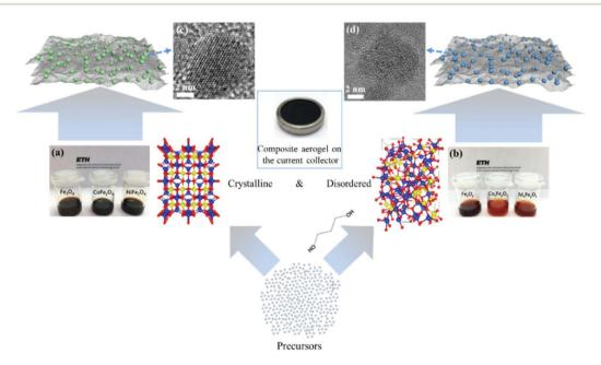
Fig. 10 Schematic of the preparation of crystalline and structurally disordered composite aerogels. Reproduced with permission from ref. 104. Copyright 2018, American Chemical Society.
