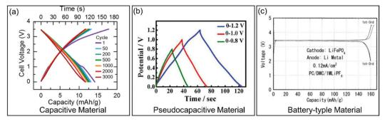
Fig. 3 Galvanostatic charge/discharge curves for different types of electrode materials. (a) Carbon-based EC material. Reproduced with permission from ref. 36. Copyright 2017, Electrochemical Society. (b) Pseudocapacitive K<sub>x</sub>MnO<sub>2</sub>. Reproduced with permission from ref. 37. Copyright 2016, American Chemical Society. (c) Battery-type LiFePO<sub>4</sub>. Reproduced with permission from ref. 38. Copyright 2001, Electrochemical Society.
