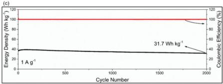
Fig. 11 (a) Voltammetric response of G-ZVO with separation between total current and pseudocapacitive current at a scan rate of 1 mV s<sup>-1</sup>. (b) Schematic of the G-ZVO||OM-HSTC hybrid device. (c) Long-term cycling stability performance of the G@ZVO||OM-HSTC hybrid device at 1.5 mA cm<sup>-2</sup>. Reproduced with permission from ref. 106. Copyright 2018, Wiley-VCH.
