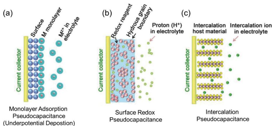
**Fig. 2** Different types of reversible redox mechanisms that give rise to pseudocapacitance: (a) monolayer adsorption pseudocapacitance (underpotential deposition), (b) surface redox pseudocapacitance, and (c) intercalation pseudocapacitance. Reproduced with permission from ref. 20. Copyright 2018, Wiley-VCH.
