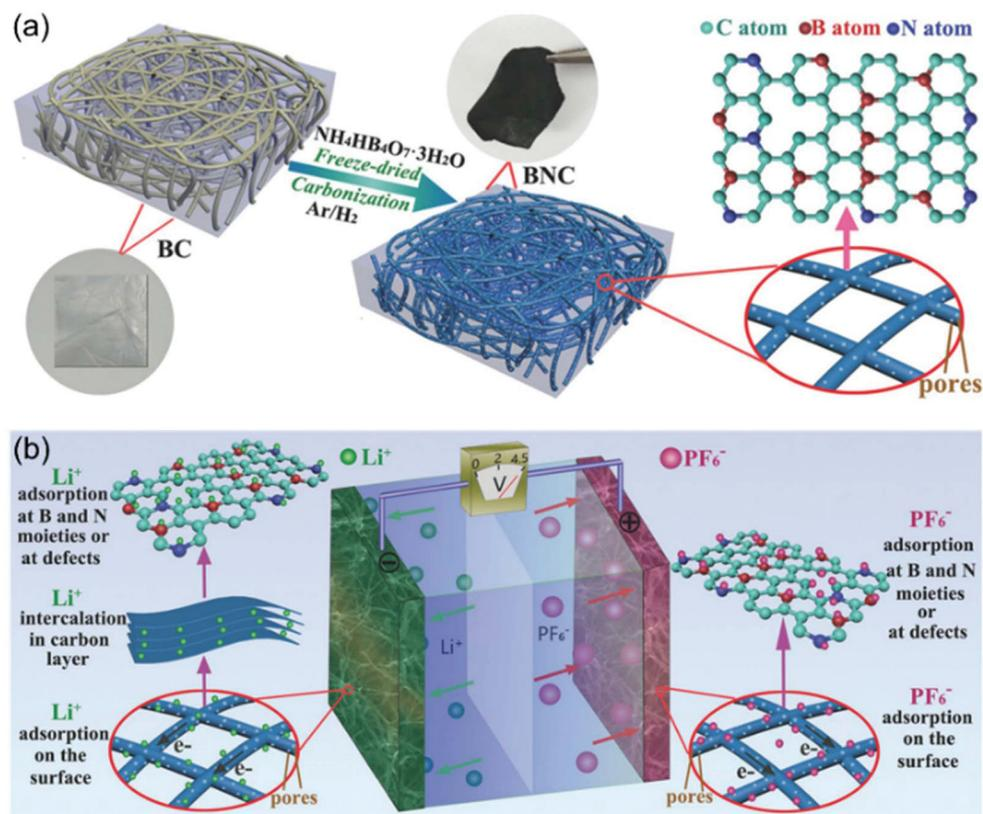
**Fig. 9** Example of an advanced non-aqueous hybrid capacitor: A LIC using B and N dual-doped carbon nanofibers as both the cathode and the anode. (a) Schematic of the fabrication process of BNC. (b) Schematic of the charge-storage mechanisms of BNC//BNC LIC. Reproduced with permission from ref. 100. Copyright 2017, Wiley-VCH.
