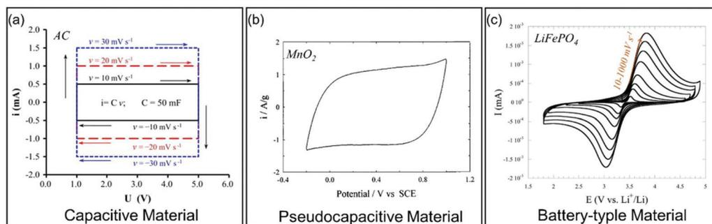
**Fig. 4** Galvanostatic charge/discharge curves for different types of electrode materials. (a) Carbon-based EC material. Reproduced with permission from ref. 39. Copyright 2013, Elsevier. (b) Pseudocapacitive  $MnO_2$ . Reproduced with permission from ref. 41. Copyright 1999, Elsevier. (c) Battery-type  $LiFePO_4$ . Reproduced with permission from ref. 40. Copyright 2011, Electrochemical Society.
