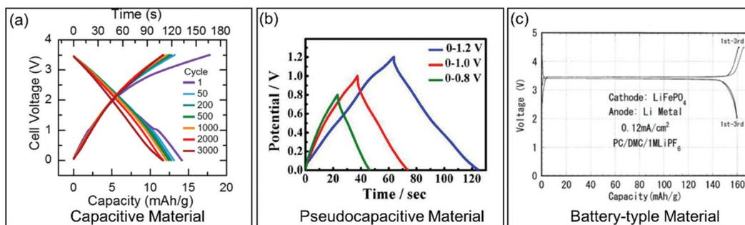
**Fig. 3** Galvanostatic charge/discharge curves for different types of electrode materials. (a) Carbon-based EC material. Reproduced with permission from ref. 36. Copyright 2017, Electrochemical Society. (b) Pseudocapacitive  $K_xMnO_2$ . Reproduced with permission from ref. 37. Copyright 2016, American Chemical Society. (c) Battery-type  $LiFePO_4$ . Reproduced with permission from ref. 38. Copyright 2001, Electrochemical Society.
