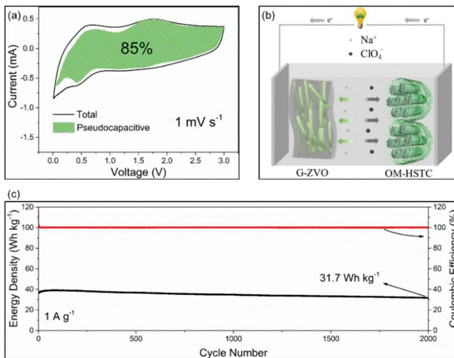
**Fig. 11** (a) Voltammetric response of G-ZVO with separation between total current and pseudocapacitive current at a scan rate of  $1 \text{ mV s}^{-1}$ . (b) Schematic of the G-ZVO||OM-HSTC hybrid device. (c) Long-term cycling stability performance of the G@ZVO||OM-HSTC hybrid device at  $1.5 \text{ mA cm}^{-2}$ . Reproduced with permission from ref. 106. Copyright 2018, Wiley-VCH.
