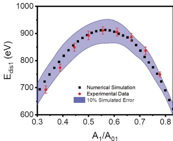
**Fig. 7** Comparison between numerical simulations and experiments on a LDPE polymer sample. The numerical simulation was performed for a 3D  $K$ - $V$  with parameters:  $E_{\text{eff}} = 111$  MPa;  $\eta_{\text{com}} = 38$  Pa s. The shaded region shows the values for the dissipated energy if the viscosity coefficient is determined with a 10% relative error. The parameters used for the simulation are listed in Fig. 4.
