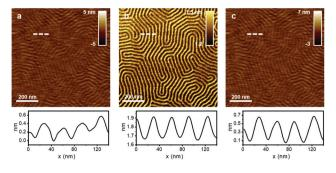
Fig. 5 Apparent, deformation and true topography of a PS-b-PMMA block co-polymer. (a) Apparent topography. (b) Deformation. (c) True topography. The bottom panels show the cross-sections across the dashed lines marked in the top panels.  $A_{01} = 90$  nm,  $A_1 = 55$  nm,  $f_{01} = 77.250$  kHz,  $k_1 = 3.2$  N m<sup>-1</sup>,  $Q_1 = 206$ ,  $A_2 = 1.3$  nm,  $f_{02} = 490.283$  kHz,  $k_2 = 166$  N m<sup>-1</sup>, R = 2 nm.
