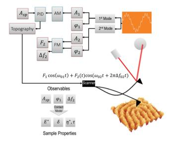
Fig. 1 Scheme of bimodal AM-FM for mapping viscoelastic properties. The microcantilever is driven simultaneously at the first two flexural resonances. An amplitude modulation feedback (AM) acting on the first mode is used to track the sample topography. A frequency modulation feedback (FM) acting on the second mode provides spatial variations of the frequency shift  $\Delta f_2$ . A theoretical model transforms the observables into the viscoelastic parameters of the tip-sample interaction force.
