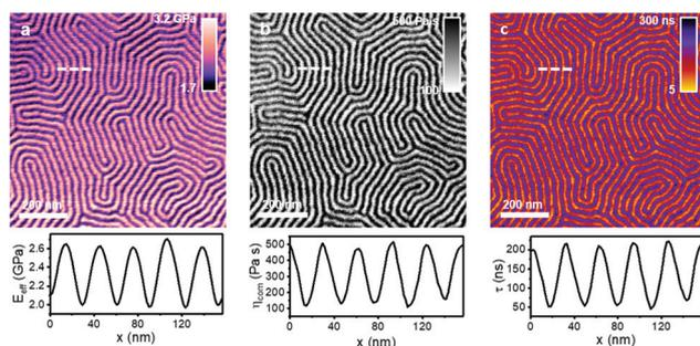
**Fig. 6** Nanomechanical maps of a PS-*b*-PMMA block co-polymer. (a) Young's modulus. (b) Viscosity coefficient. (c) Retardation time. The stiffer domains (PMMA) show a lower viscosity coefficient and a faster response time. The bottom panels show the cross-sections across the lines marked in the top panels. The above images have been obtained simultaneously with those of Fig. 5. A tip radius of 2 nm has been used to deduce the parameters.
