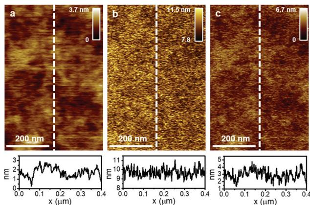
**Fig. 2** Apparent, deformation and true topography of a polymer blend. (a) Apparent topography. (b) Deformation. (c) True topography. The bottom panels show the cross-sections across the lines marked in the top panels. The measurement parameters are  $A_{01} = 87$  nm,  $A_1 = 51$  nm,  $f_{01} = 324.783$  kHz,  $k_1 = 43.2$  N m<sup>-1</sup>,  $Q_1 = 532$ ,  $A_2 = 0.5$  nm,  $f_{02} = 2009$  kHz,  $k_2 = 2269$  N m<sup>-1</sup>,  $R = 11$  nm.
