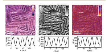
Fig. 6 Nanomechanical maps of a PS-b-PMMA block co-polymer. (a) Young's modulus. (b) Viscosity coefficient. (c) Retardation time. The stiffer domains (PMMA) show a lower viscosity coefficient and a faster response time. The bottom panels show the cross-sections across the lines marked in the top panels. The above images have been obtained simultaneously with those of Fig. 5. A tip radius of 2 nm has been used to deduce the parameters.
