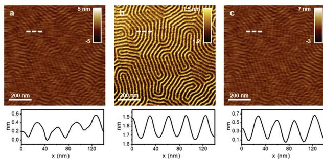
**Fig. 5** Apparent, deformation and true topography of a PS-*b*-PMMA block co-polymer. (a) Apparent topography. (b) Deformation. (c) True topography. The bottom panels show the cross-sections across the dashed lines marked in the top panels.  $A_{01} = 90$  nm,  $A_1 = 55$  nm,  $f_{01} = 77.250$  kHz,  $k_1 = 3.2$  N m $^{-1}$ ,  $Q_1 = 206$ ,  $A_2 = 1.3$  nm,  $f_{02} = 490.283$  kHz,  $k_2 = 166$  N m $^{-1}$ ,  $R = 2$  nm.
