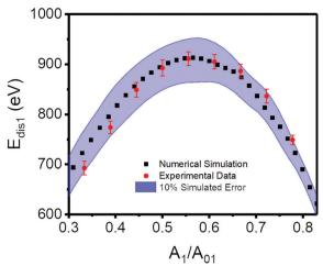
Fig. 7 Comparison between numerical simulations and experiments on a LDPE polymer sample. The numerical simulation was performed for a 3D K–V with parameters:  $E_{\rm eff}$  = 111 MPa;  $\eta_{\rm com}$  = 38 Pa s. The shaded region shows the values for the dissipated energy if the viscosity coefficient is determined with a 10% relative error. The parameters used for the simulation are listed in Fig. 4.
