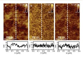
Fig. 2 Apparent, deformation and true topography of a polymer blend. (a) Apparent topography. (b) Deformation. (c) True topography. The bottom panels show the cross-sections across the lines marked in the top panels. The measurement parameters are  $A_{01}=87$  nm,  $A_{1}=51$  nm,  $f_{01}=324.783$  kHz,  $k_{1}=43.2$  N m<sup>-1</sup>,  $Q_{1}=532$ ,  $A_{2}=0.5$  nm,  $f_{02}=2009$  kHz,  $k_{2}=2269$  N m<sup>-1</sup>, R=11 nm.
