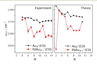
Fig. 9 Measured and calculated CO stretching frequencies,  $\nu_{\text{CO}}$ , for the first adsorbed CO molecule on  $\text{Au}_{N}^{+}$  and  $\text{PdAu}_{N-1}^{+}$  clusters.
