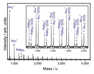
Fig. 2 Typical mass spectrum of  $Au_N^+$  and  $PdAu_{N-1}^+$  clusters and their CO complexes, formed in the low-pressure collision reaction cell. Clusters are exposed to a CO gas pressure of  $P_{CO}$  = 0.2 Pa. The inset shows a zoom-in for N = 7-10.
