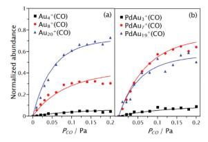
Fig. 5 Normalized abundances of  $Au_4^+(CO)$ ,  $Au_8^+(CO)$  and  $Au_{20}^+(CO)$ in (a) and PdAu<sub>3</sub><sup>+</sup>(CO), PdAu<sub>7</sub><sup>+</sup>(CO) and PdAu<sub>19</sub><sup>+</sup>(CO) in (b), as a function of  $P_{CO}$  at the reaction cell. Points represent the experimental data, while solid lines are fits with eqn (2).
