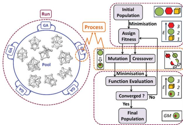
**Fig. 1** Schematic representation of the BPGA programme. The left side shows the pool methodology, containing the structural database (within the blue circle) and defines the run (purple colour), and process (orange colour) concepts. The instance concept consists of carrying out the specified type of mutation or crossover (process), followed by DFT local minimization. The flow chart on the right side illustrates the GA operations.
