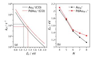
Fig. 7 (a) Dissociation rates as a function of the critical energy, simulated by RRKM theory for N=8. Dotted lines represent the intersection between the measured dissociation rates and the corresponding critical energy. (b) CO binding energies extracted by the RRKM analysis based on the experimental  $k_{\rm d}$  rates.
