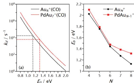
Fig. 7 (a) Dissociation rates as a function of the critical energy, simulated by RRKM theory for  $N = 8$ . Dotted lines represent the intersection between the measured dissociation rates and the corresponding critical energy. (b) CO binding energies extracted by the RRKM analysis based on the experimental  $k_d$  rates.
