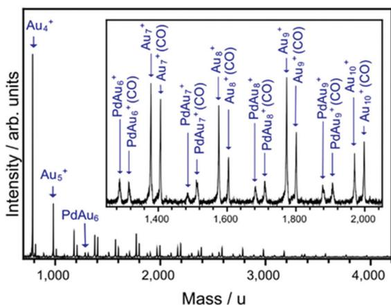
Fig. 2 Typical mass spectrum of  $\text{Au}_N^+$  and  $\text{PdAu}_{N-1}^+$  clusters and their CO complexes, formed in the low-pressure collision reaction cell. Clusters are exposed to a CO gas pressure of  $P_{\text{CO}} = 0.2$  Pa. The inset shows a zoom-in for  $N = 7-10$ .
