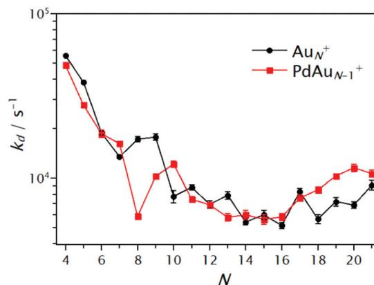
Fig. 6 Dissociation rates of CO for  $Au_N^+(CO)$  (black circles) and  $PdAu_{N-1}^+(CO)$  (red squares) clusters extracted by fitting eqn (2) to the normalized abundance curves as a function of  $P_{CO}$ .
