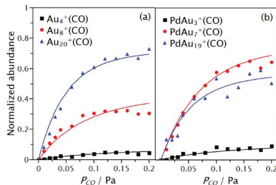
Fig. 5 Normalized abundances of  $Au_4^+(CO)$ ,  $Au_8^+(CO)$  and  $Au_{20}^+(CO)$  in (a) and  $PdAu_3^+(CO)$ ,  $PdAu_7^+(CO)$  and  $PdAu_{19}^+(CO)$  in (b), as a function of  $P_{CO}$  at the reaction cell. Points represent the experimental data, while solid lines are fits with eqn (2).
