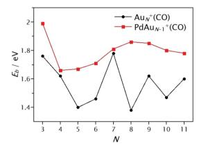
Fig. 4 Cluster-CO binding energies  $(E_{\rm b})$  calculated by DFT as a function of cluster size for  $Au_N^+(CO)$  (N = 3-11) and  $PdAu_{N-1}^+(CO)$  (N = 3-10).
