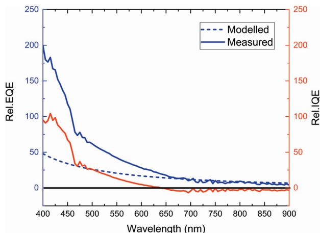
**Fig. 4** Relative enhancement in IQE (red solid line) and EQE (blue solid line) after deposition of a 32 nm thick QD layer. The blue dashed line is the modelled EQE enhancement due to antireflection. The EQE and IQE spectral responses shown were measured without light bias.
