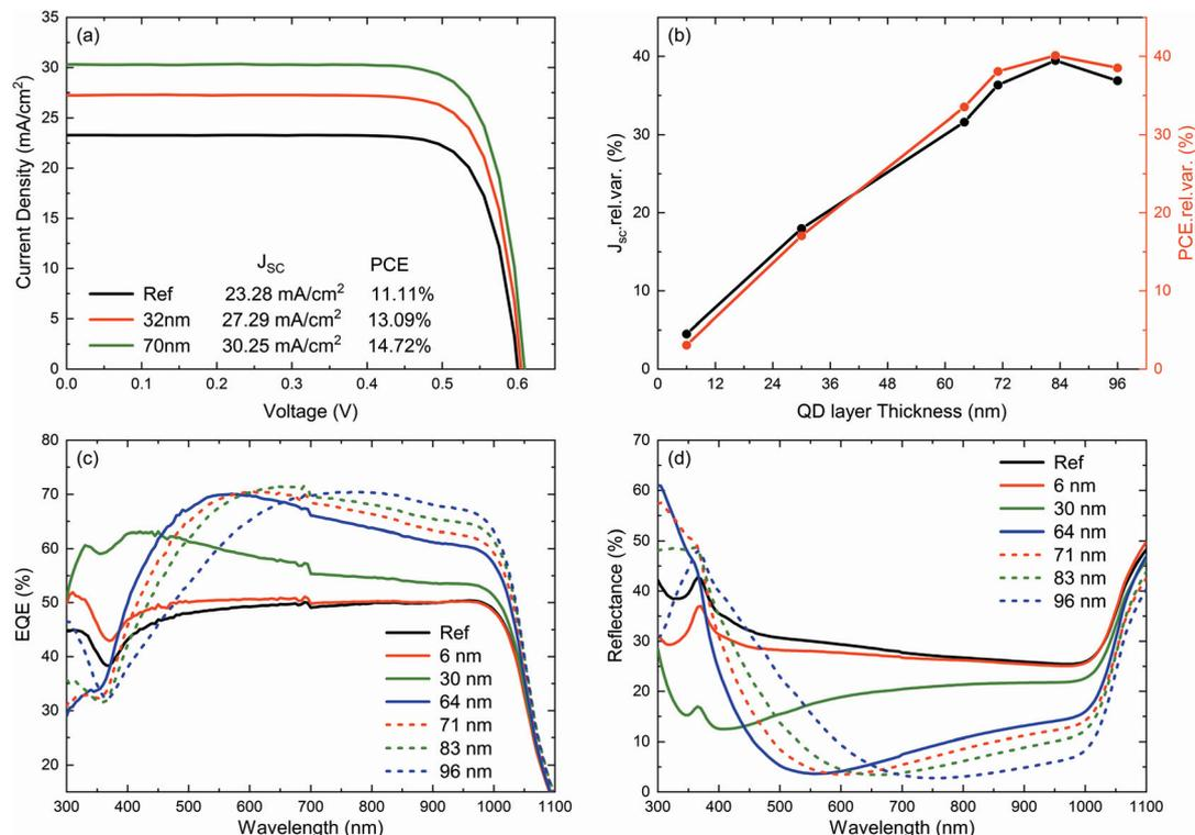
**Fig. 3** (a)  $J$ - $V$  curves of the IBC solar cell before and after hybridization of our best device. (b) Relative variations of short-circuit current ( $J_{sc}$ ) and power conversion efficiency (PCE) of the solar cell for different QD layer thicknesses. (c) EQE of hybrid IBC solar cells for different QD layer thicknesses. (d) Reflectance of the hybrid IBC solar cell for different thicknesses of QDs. The EQE shown here was measured under 1 sun light bias.
