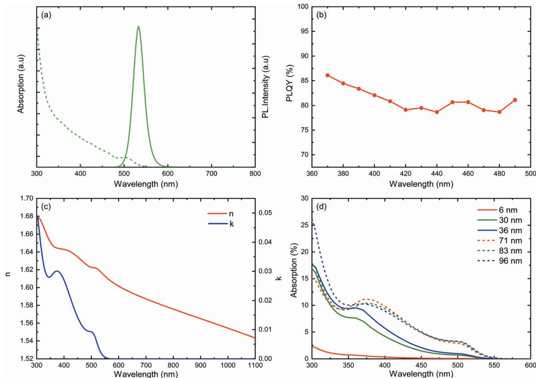
**Fig. 2** (a) Absorption (dashed line) and photoluminescence (solid line) of  $\text{CdSe}_{1-x}\text{S}_x/\text{ZnS}$  QDs deposited on a glass slide, (b) measured PLQY of  $\text{CdSe}_{1-x}\text{S}_x/\text{ZnS}$  QDs in solution for a concentration of  $0.16 \text{ mg ml}^{-1}$ , (c) optical constants of  $\text{CdSe}_{1-x}\text{S}_x/\text{ZnS}$  QDs, and (d) modelled absorption for different thicknesses of the QD layer on Si.
