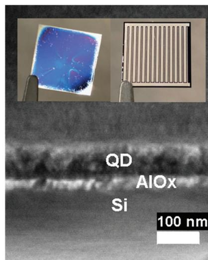
**Fig. 1** (a) Schematic representation of the hybrid planar IBC solar cell and (b) the cross-sectional SEM image of QDs and AlO<sub>x</sub> on the IBC solar cell, where the inset photo shows the front and rear of the cell.
