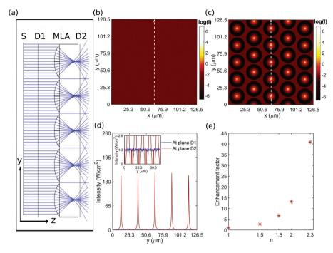
Fig. 4 (a) Geometry used in the ray-tracing simulations. Simulated excitation light intensity distribution (b) before and (c) at the right edge of the MLA. (d) Line profile analyses of excitation light intensity along the selected lines indicated by white lines in (b) and (c). (e) Calculated enhancement factors for upconversion emission bands with different slope factors.
