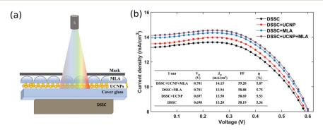
Fig. 5 (a) Schematic illustration of the configuration of UCNP- and/or MLA-enhanced DSSC. S – source (b) the current density–voltage (J-V) characteristics of DSSC, DSSC + UCNP, DSSC + MLA and DSSC + UCNP + MLA under AM1.5 G light irradiation (0.1 W cm<sup>-2</sup>).
