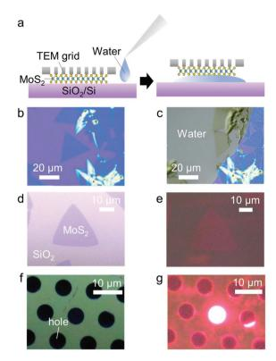
Fig. 1 (a) Schematic summarizing the preparation of a suspended sample on a TEM grid via water-aided transfer. Optical microscopy images showing a MoS<sub>2</sub> monolayer grown on a SiO<sub>2</sub>/Si substrate (b) before and (c) after water casting. Optical microscopy and PL images of MoS<sub>2</sub> monolayers (d, e) grown on a SiO<sub>2</sub>/Si substrate and (f, g) suspended on a TEM grid, respectively.
