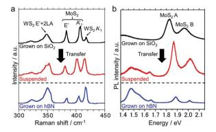
Fig. 4 (a) Raman and (b) PL spectra obtained from CVD-grown MoS<sub>2</sub>/ WS<sub>2</sub> heterostructures supported on a SiO<sub>2</sub>/Si substrate and suspended in air. The spectra of a MoS<sub>2</sub>/WS<sub>2</sub> heterostructure grown directly on an hBN surface is also shown for comparison. The spectra have been vertically shifted for clarity.
