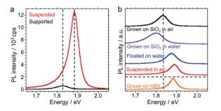
Fig. 2 (a) PL spectra of a  $MoS_2$  monolayer suspended on a TEM grid and on a  $SiO_2/Si$  support. Broken lines indicate the primary peak position for each sample. (b) Normalized PL spectra of a  $MoS_2$  monolayer on a  $SiO_2/Si$  substrate in air and water, together with those of substrate-free samples floating on water and suspended in air, as well as that of a  $MoS_2$  monolayer grown directly on an hBN surface. The spectra have been vertically shifted for clarity.
