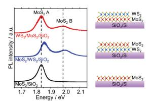
Fig. 5 PL spectra and structure models for (bottom) a MoS<sub>2</sub> monolayer grown directly on a SiO<sub>2</sub>/Si substrate, (center) a WS<sub>2</sub> monolayer covered by a MoS<sub>2</sub> monolayer, and (upper) a MoS<sub>2</sub> monolayer covered by a WS<sub>2</sub> monolayer.
