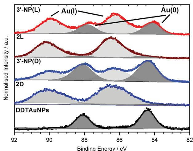
**Fig. 4** Normalised Au 4f XPS narrow scan spectra of 3'-NP(D/L) NHC-AuNPs and the 2(D/L) complex. Raw data are shown as coloured scatter plots. Deconvolutions are shown in grey, resulting envelopes in colour.
