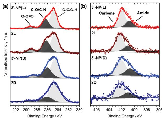
**Fig. 3** Normalised C 1s (a) and N 1s (b) XP spectra of 3'-NP(D/L) NHC-AuNPs and the 2(D/L) complexes. Raw data are shown as coloured scatter plots. Deconvolutions are shown in grey, resulting envelopes in colour.
